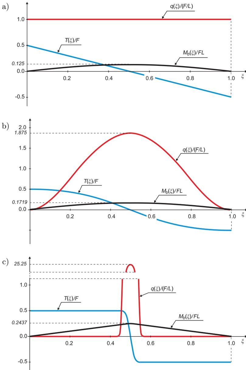
FIG. 3. The example diagrams of the intensity of the load (2.5), shear force (2.6) and bending moment (2.7): a) for  $n = 0$  – the uniformly distributed load, b) for  $n = 2$  – the non-uniformly distributed load, c) for  $n = 500$  – the load approximating the three-point bending.
