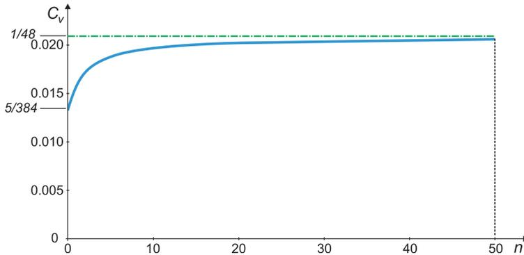
FIG. 6. Graph of the deflection coefficient  $C_v$  as a function of the natural number  $n$ .
