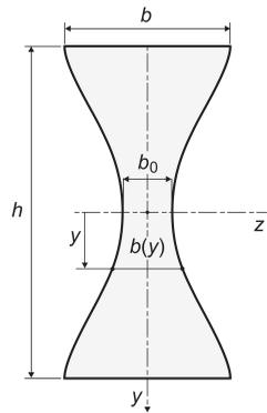
FIG. 1. Scheme of the bisymmetrical cross-section of the beam.
