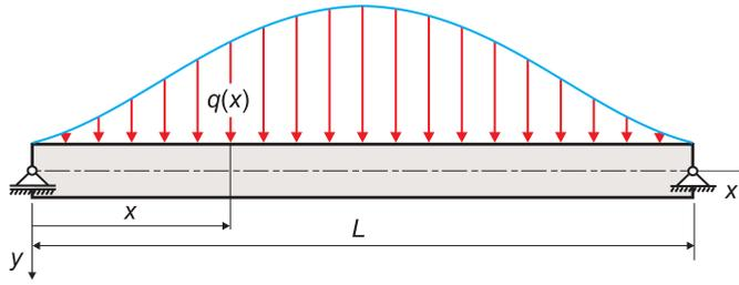
FIG. 2. Scheme of the simply-supported beam under non-uniformly distributed load.
