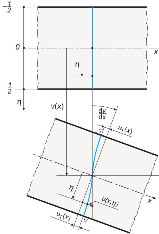
FIG. 4. Scheme of the deformation of a planar cross-section – the nonlinear hypothesis.
