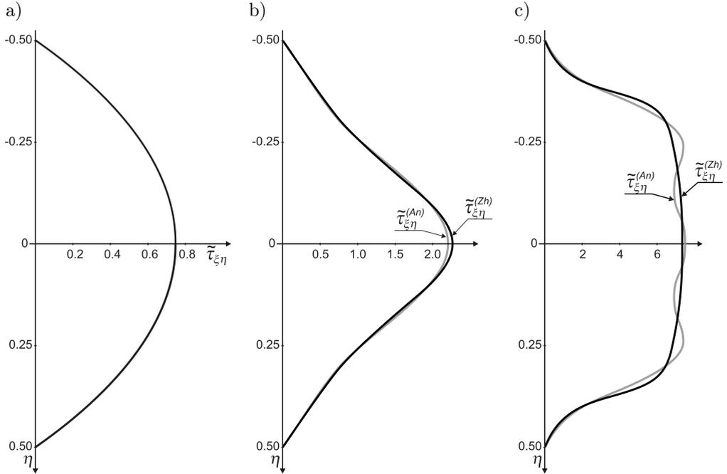
FIG. 7. Graphs of the analytical (3.14) and Zhuravsky's (3.16) shear stresses in the cross-sections: a) CS-1, b) CS-2, c) CS-3.
