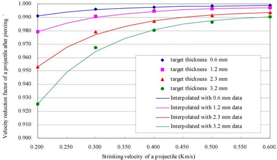
FIG. 1. Velocity reduction factors of projectile after piercing the metal plate.
