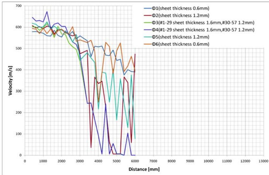
FIG. 14. Distance-velocity data using 40 mm rifled gun.
