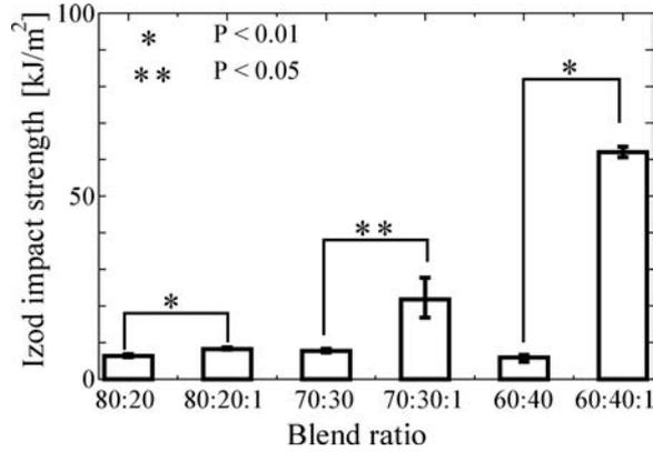
FIG. 4. Impact resistance of different PLA/PBAT alloys.
