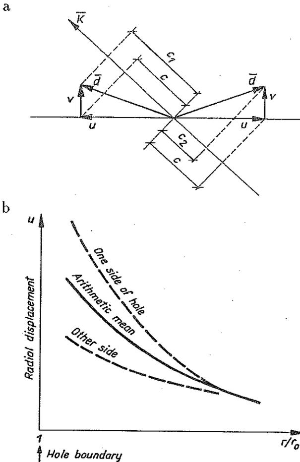
FIG. 4. Geometrical interpretation of the principle of measuring surface displacements.
