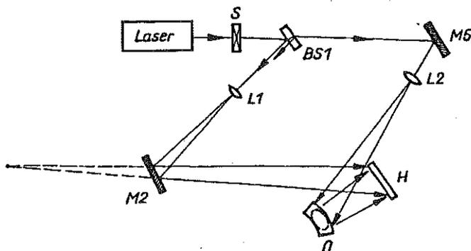
FIG. 1. Hologram registering system: *S* - shutter, *BS1* - beam splitter, *M2*, *M5* - reflecting mirrors, *L1*, *L2* - microscopic lens, *O* - object, *H* - holographic plate.
