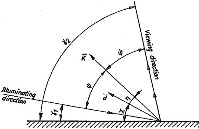
FIG. 2. Displacement components in the plane of interferometer.  $\vec{d}$  - displacement vector,  $\vec{K}$  - sensitivity vector of the holointerferogram.
