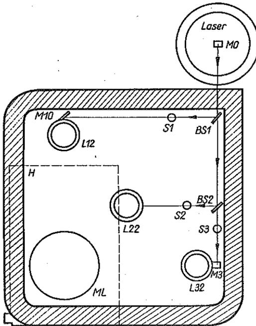
FIG. 7. View of the front side of the camera. Laser light beam is split among 3 interferometers I1, I2, I3. *M* – mirrors, *BS* – beam splitters, *L* – microscopic lenses, *ML* – magnifying lens, *S* – shutters, *H* – holographic plate.
