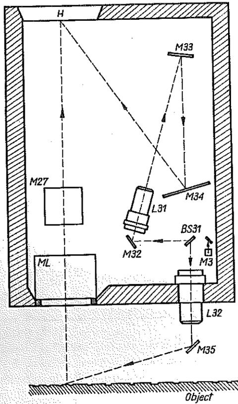
FIG. 8. Set-up of interferometer I3. *M* – mirrors, *BS* – beam splitters, *L* – microscopic lenses, *ML* – magnifying lens, *H* – holographic plate.
