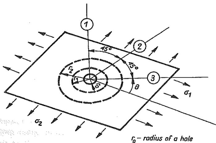
FIG. 5. Directions of measured displacements in the holointerferograms.
