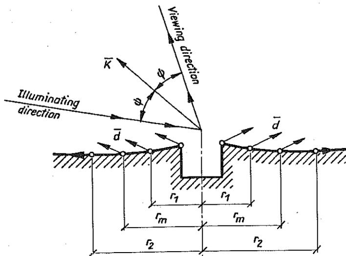
FIG. 3. Deformations around a hole.
