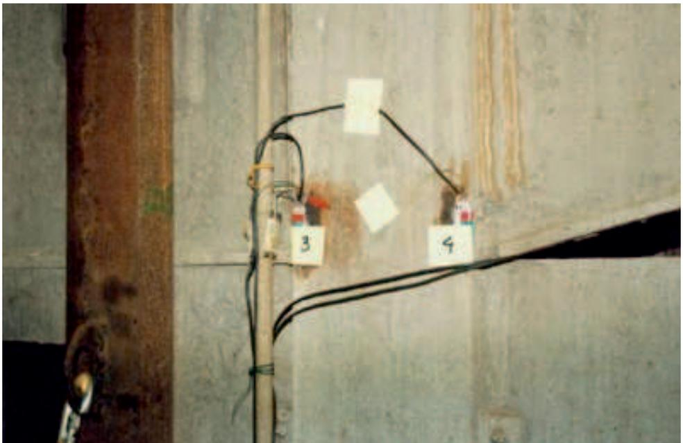
FIG. 23. Strain gauges TC3 and TC4 fixed to the mid-point string, at the attachment point to the head structure.
