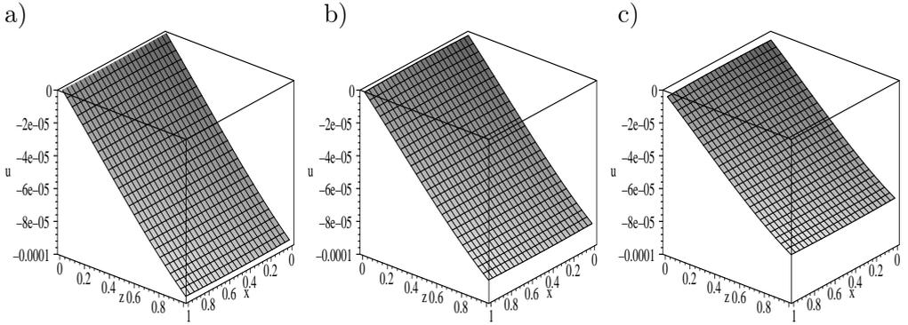
FIG. 8. Approximation of displacement  $u_z(x, 0.5, z, t)$  for time a)  $t = 0$ , b)  $t = 0.0001$ , c)  $t = 0.00016$ .
