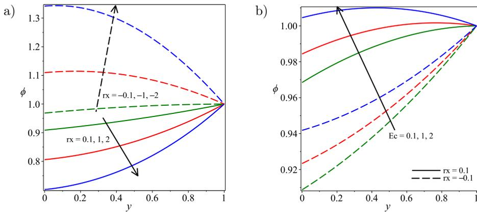
FIG. 12. Steady-state concentration profiles with increasing  $rx$  ( $rx < 0$ ,  $rx > 0$ ) (a) and  $Ec$ ,  $rx$  (b).
