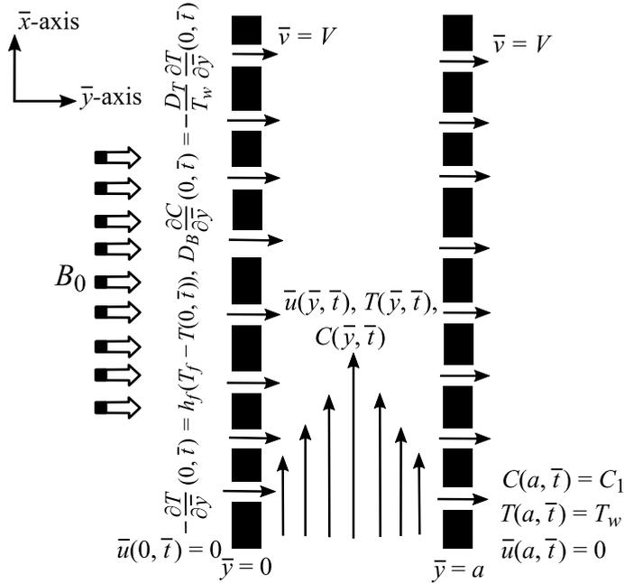
FIG. 1. Flow diagram with the coordinate system.
