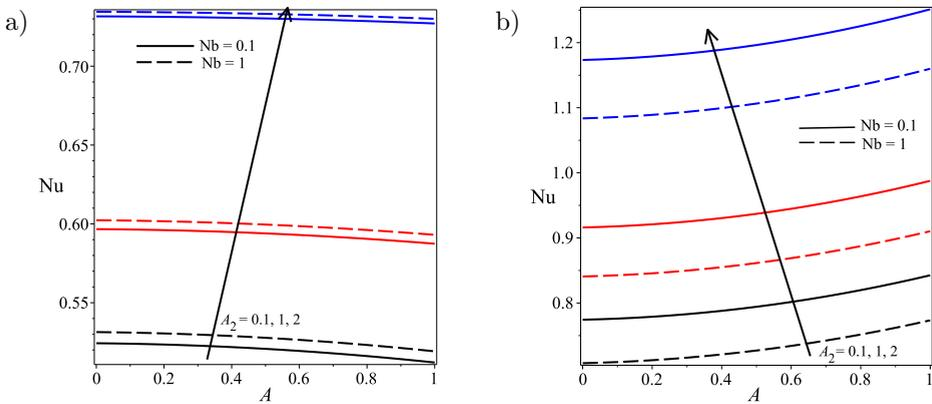
FIG. 16. Nusselt number  $Nu$  vs. pressure gradient  $A$  with increasing  $A_2$  and  $Nb$ :
