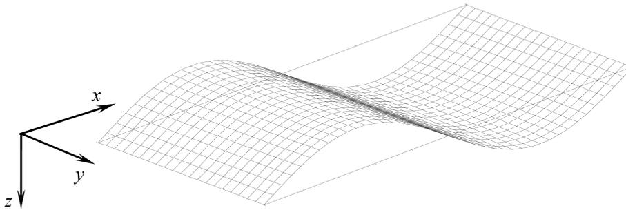
FIG. 15. The first buckling mode.
