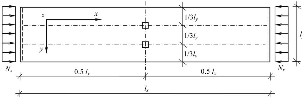
FIG. 10. The plate simply-supported on two opposite edges with two remaining free edges resting on two internal column supports under constant normal loading.
