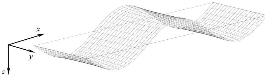
FIG. 17. The first buckling mode.
