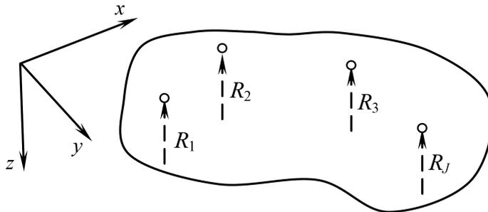
FIG. 1. A plate internally supported at selected points.
