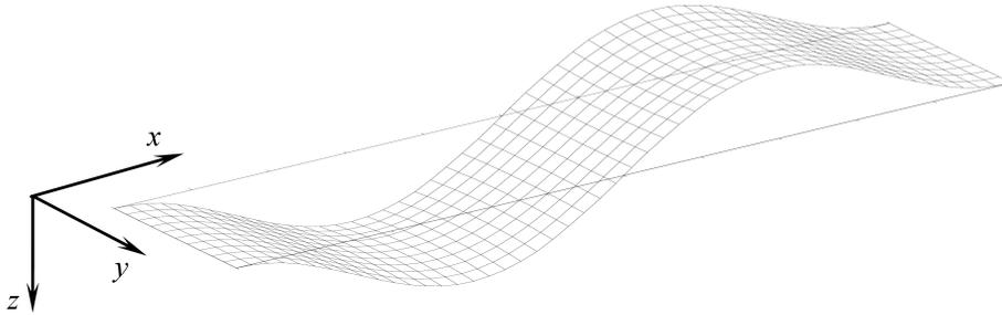
FIG. 13. The first buckling mode.
