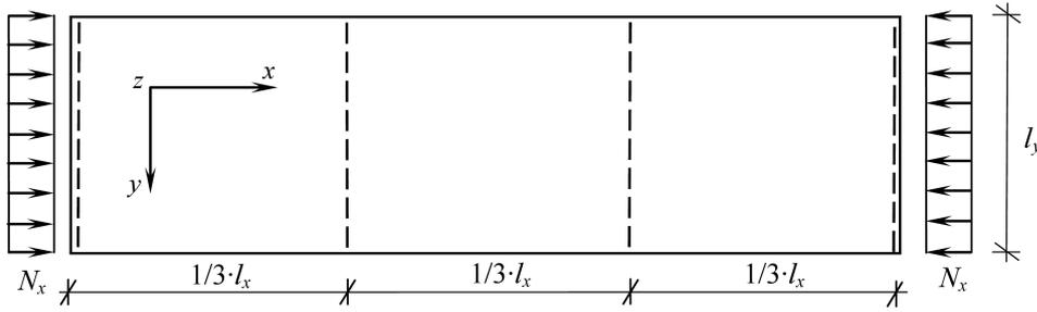
FIG. 16. The plate simply-supported on two opposite and diagonal edges resting on linear continuous internal support under constant normal loading.
