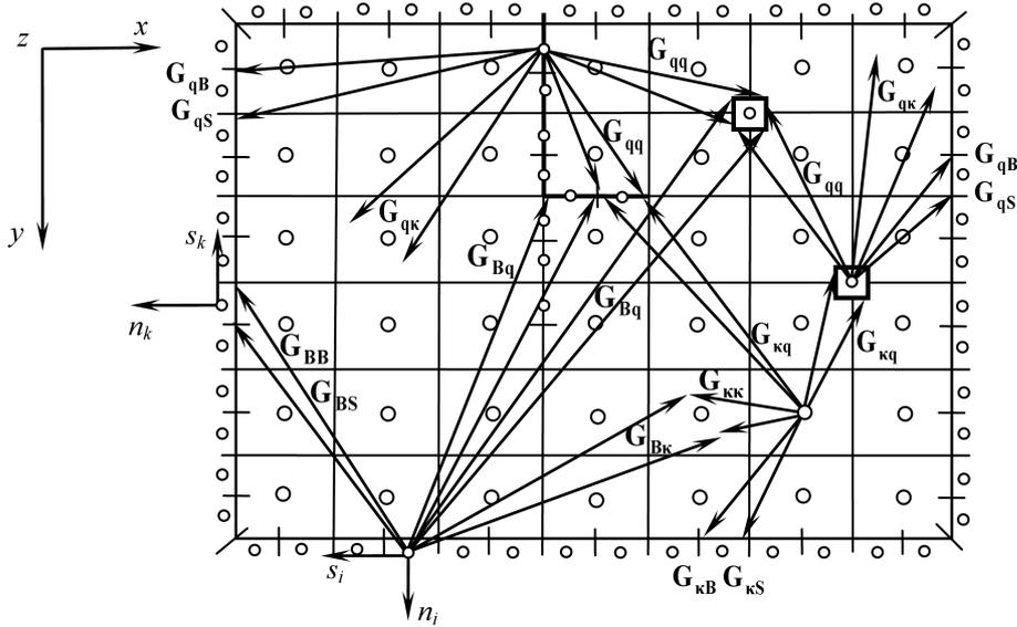
FIG. 8. Calculation of boundary and domain integrals.
