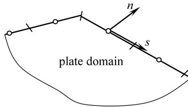
FIG. 5. Collocation point assigned to the boundary element of constant type.
