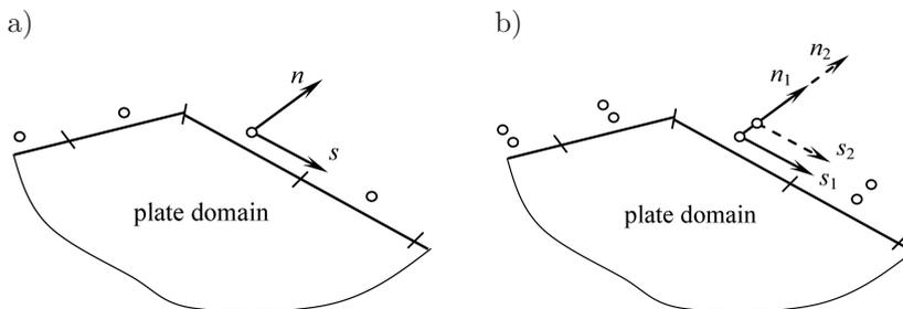
FIG. 6. a) one collocation point, b) two collocation points assigned to the boundary element of constant type.
