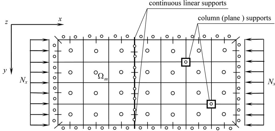
FIG. 7. Distribution of in-plane loading.
