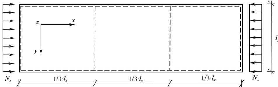
FIG. 18. The plate simply-supported on all edges resting on two linear continuous internal supports under constant normal loading.
