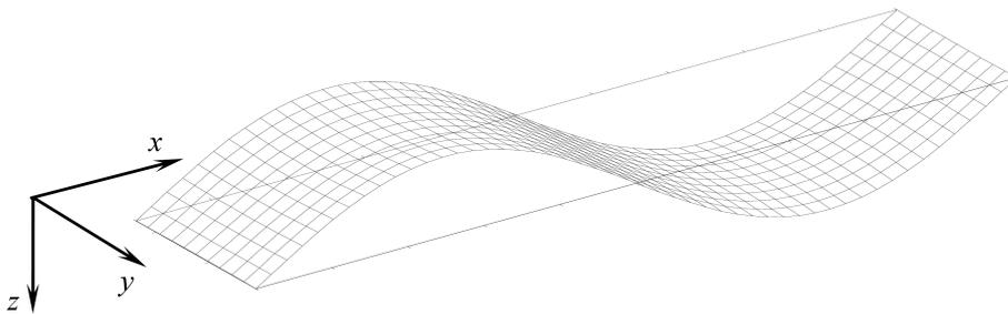
FIG. 11. The first buckling mode.
