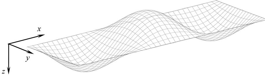
FIG. 19. The first buckling mode.
