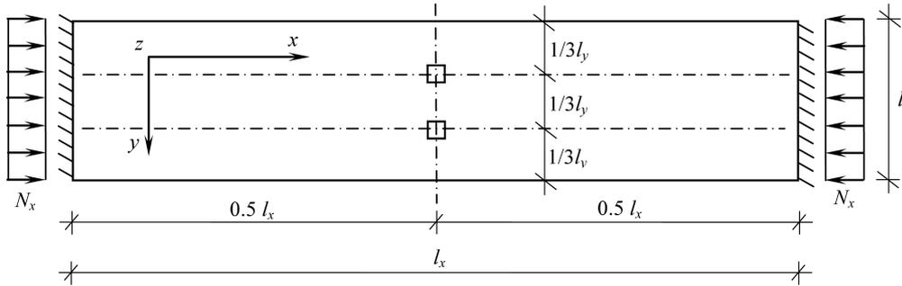
FIG. 12. The plate simply-supported on two opposite edges with two remaining free edges resting on two internal column supports under constant normal loading.
