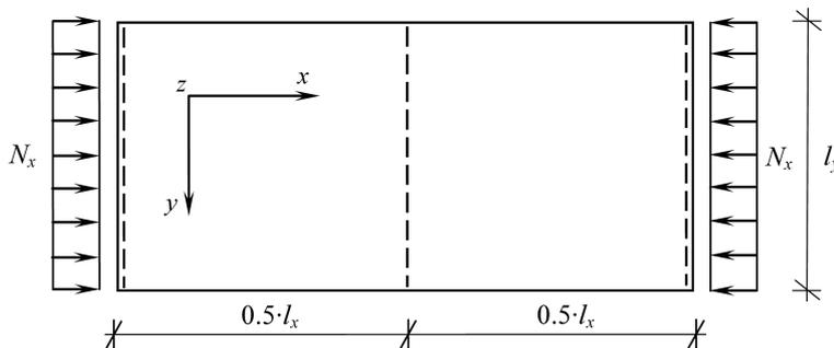
FIG. 14. The plate, simply-supported on two opposite edges with two free edges resting on internal continuous support under constant normal loading.
