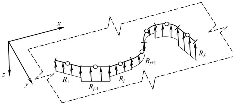
FIG. 3. A plate resting on linear continuous internal supports.
