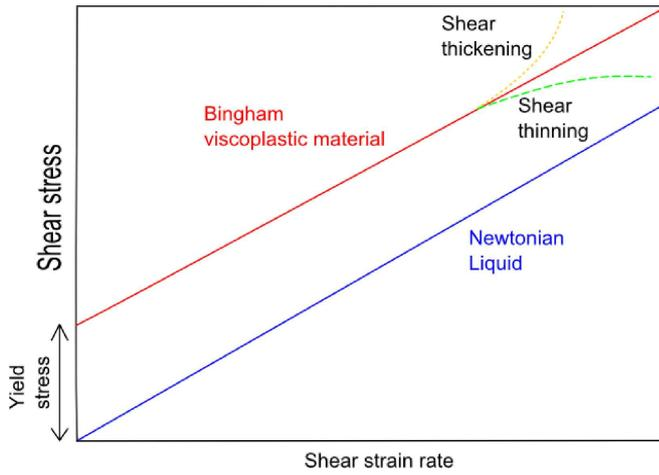
FIG. 6. Schematic view of the inadequacy of Bingham model.
