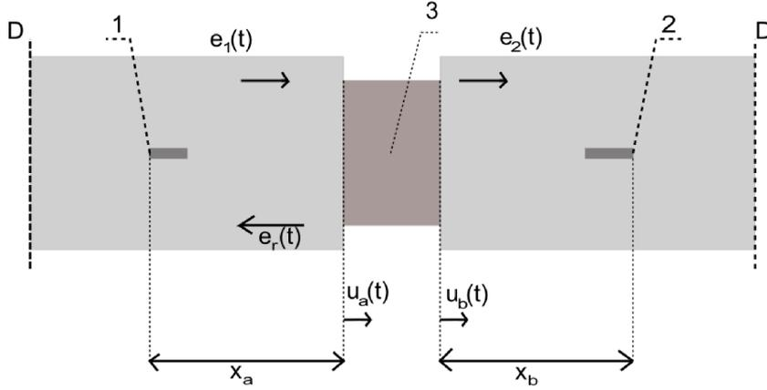
FIG. 5. Split-Hopkinson pressure bar: 1, 2) strain gauges, 3) specimen, D: bar diameter,  $e_1(t)$ : axial strain of incident wave in the bar (1),  $e_2(t)$ : axial strain of reflected wave in the bar (2),  $e_r(t)$ : axial strain of reflected wave,  $u_a(t)$  incident displacement in bar (1),  $u_b(t)$ : transmitted displacement in bar (2).
