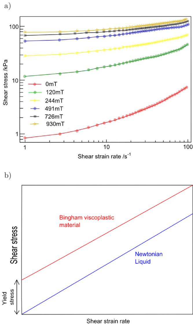
FIG. 2. Characteristics shear stress to shear strain rate [13]:
