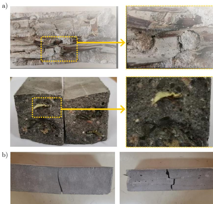
FIG. 8. Mechanism of bonding between the DPF and cement mortar (a), and the failure mode after applying flexural strength (b).
