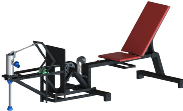
FIG. 2. Design of the newly developed pedal-operated reciprocating water pump.
