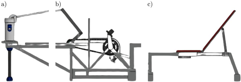
FIG. 3. Pedal-operated reciprocating pump:
