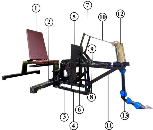
FIG. 4. Members and parts of the newly developed pedal-operated reciprocating pump.
