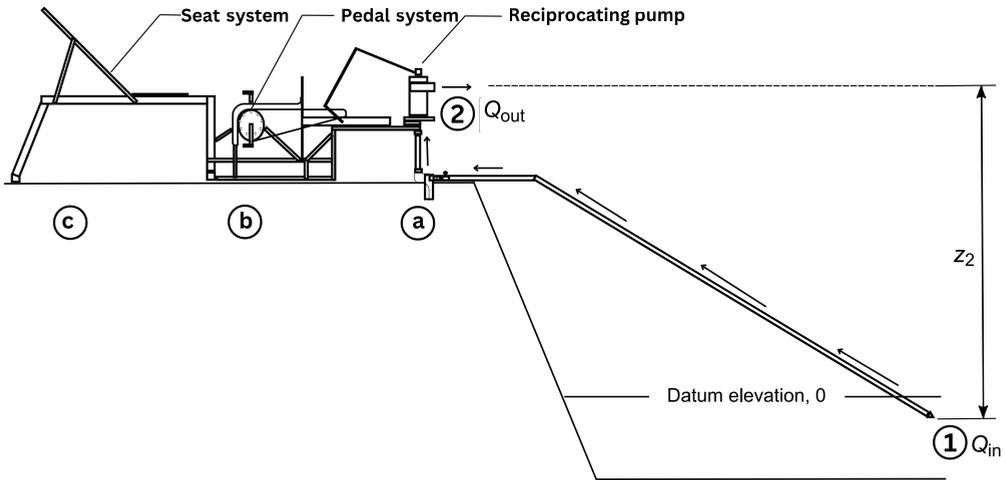
FIG. 5. Schematic diagram of the water pumping system.
