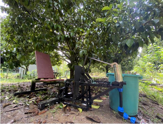
FIG. 8. Actual prototype of the newly developed pedal-operated reciprocating water pump.
