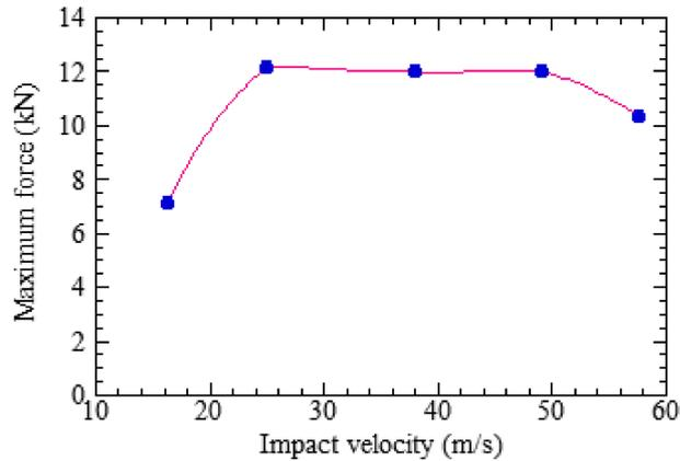
FIG. 12. Influence of the impact velocity on the rupture stress.
