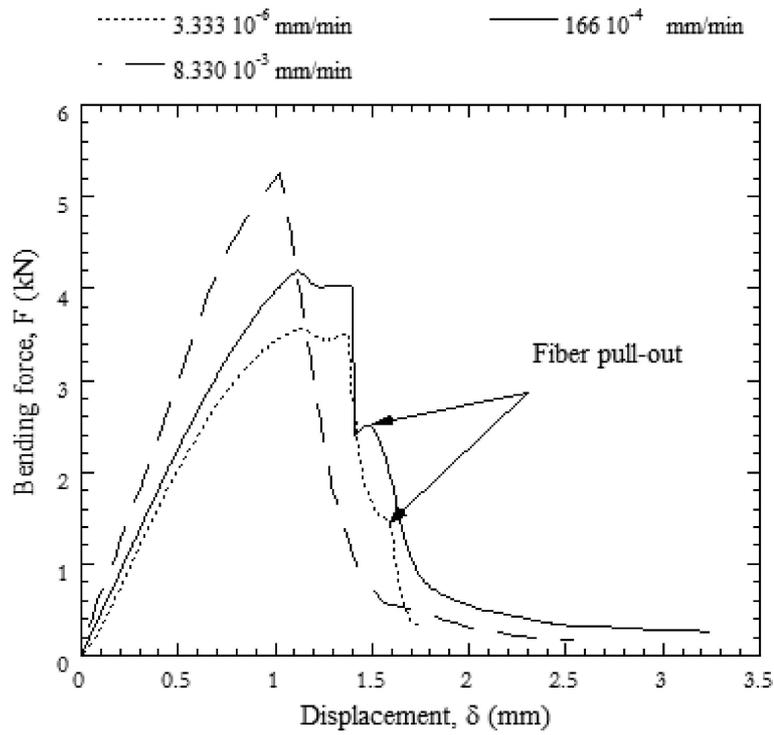
FIG. 3. Comparison of force-displacement curves for different quasi-static displacement rates.
