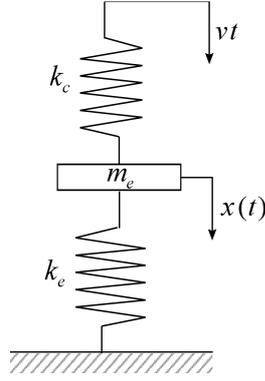
FIG. 7. Mechanical model representing behaviour of the impactor-specimen system during impact loading.
