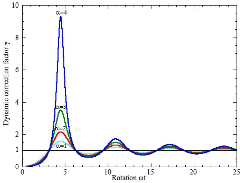
FIG. 9. Dynamic correction factor  $\gamma$  based on the Williams model for different values of  $\alpha$ .
