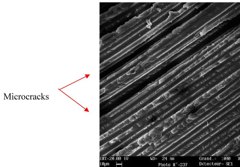
FIG. 4. Microcracks in the matrix close to the tensile face.
