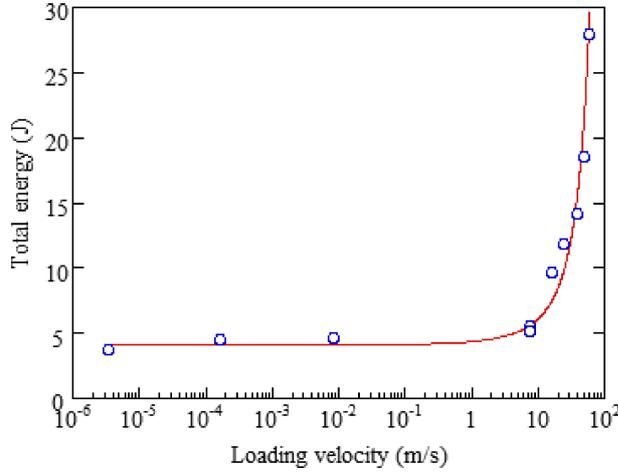
FIG. 14. Influence of the loading velocity on the total energy.
