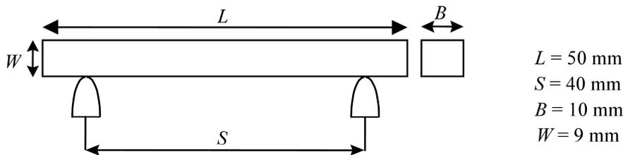
FIG. 1. Specimen geometry and schematic description of the device used for bending tests.
