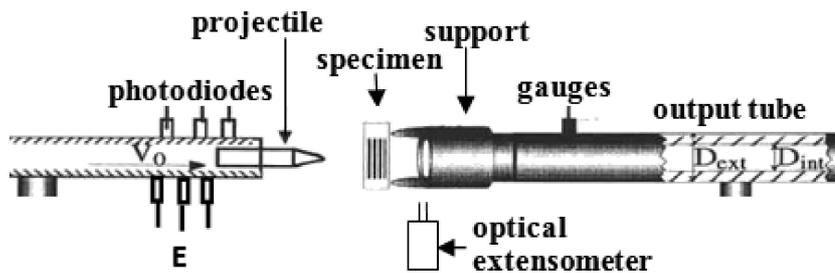
FIG. 2. Configuration for dynamic bending test [1].
