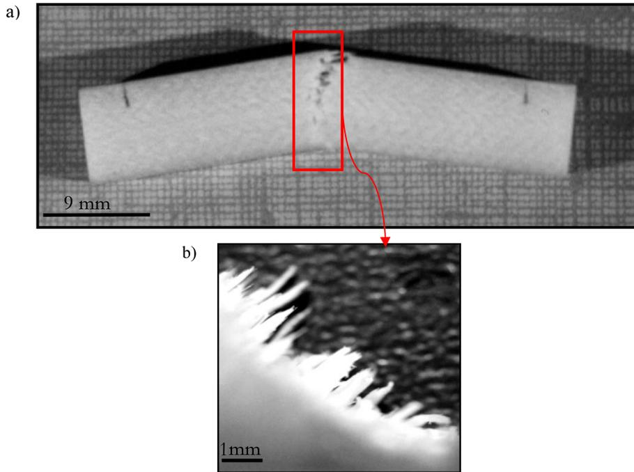
FIG. 5. a) Quasi-static rupture after three-point bending test, b) rupture face of the specimen loaded by quasi-static three-point bending.
