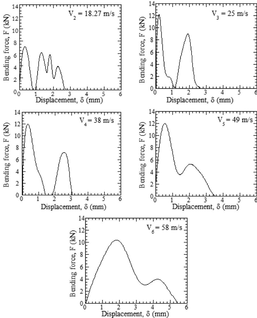
FIG. 6. Evolution of the transmitted force as a function of displacement at different impact velocities.
