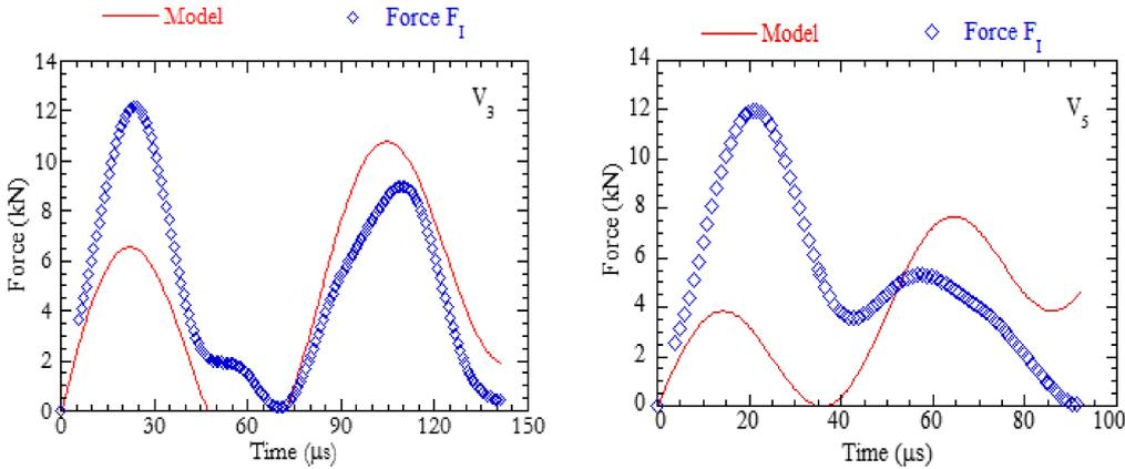
FIG. 8. Comparison between Williams model and equation; force is calculated at the impact point, the impact velocities are  $V_3 = 25$  m/s and  $V_5 = 49$  m/s.
