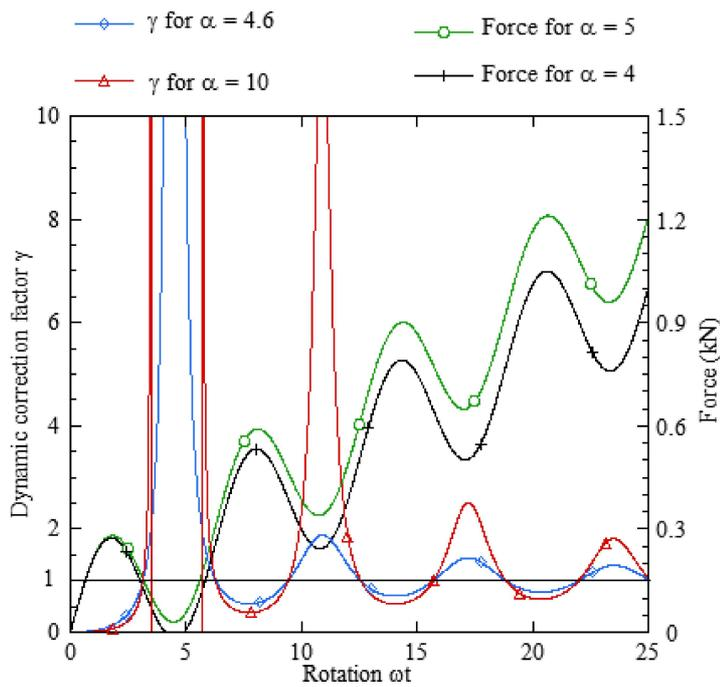
FIG. 10. Evolution of the dynamic correction factor  $\gamma$  as a function of time (Williams model);  $V_0 = 1$  m/s,  $k_e = 4.055 \cdot 10^6$  N/m,  $\omega = 80,000$  rad/s.
