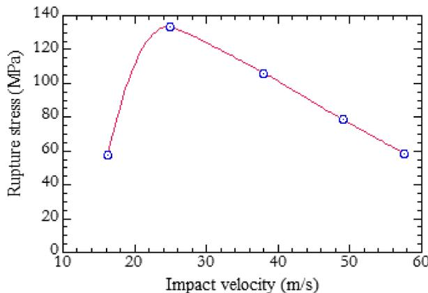
FIG. 11. Influence of the impact velocity on the rupture stress.
