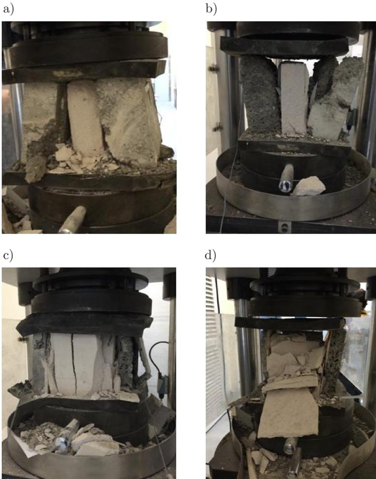
FIG. 11. Failure modes of plain and grooved sandwich specimens at different loading rates: a) GS1, b) GS2, c) PS1, d) PS2.
