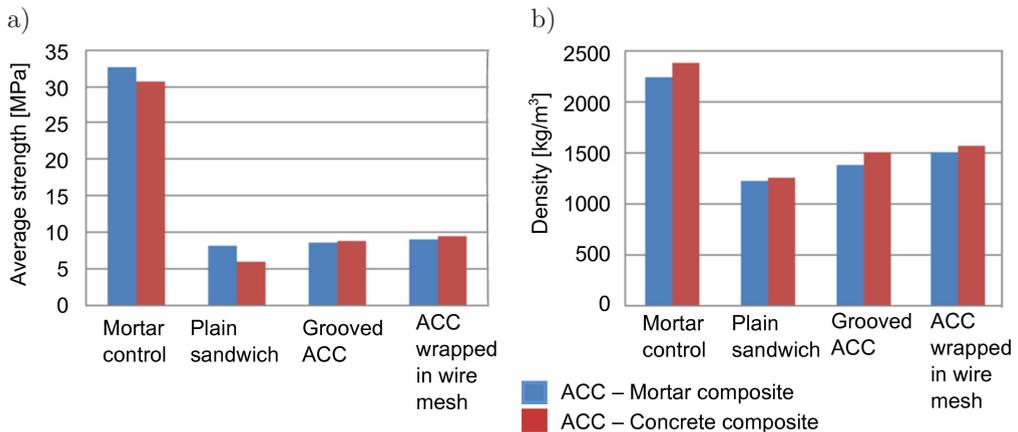
FIG. 4. Test results for the first set of composite block specimens at 7 days using a 1.8 MPa AAC: a) average strength, b) density.
