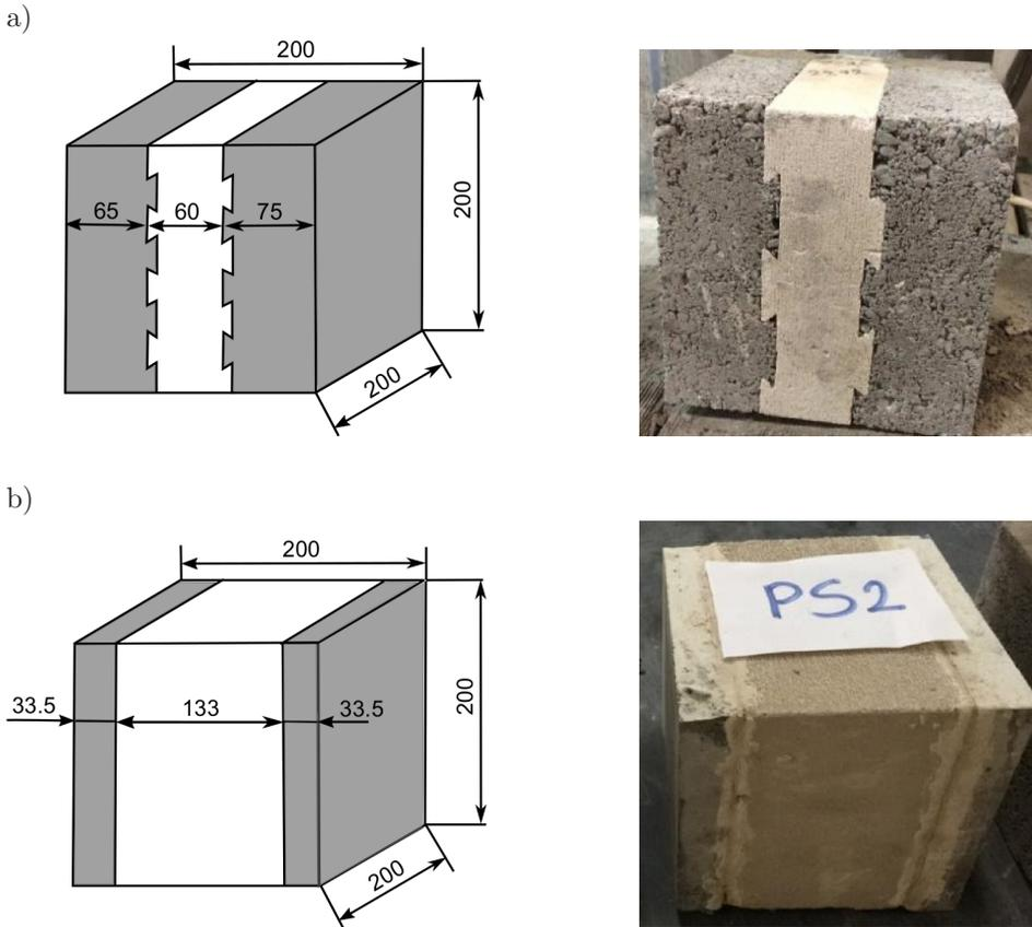
FIG. 7. Geometric description of: a) grooved sandwich, b) plain sandwich composites.
