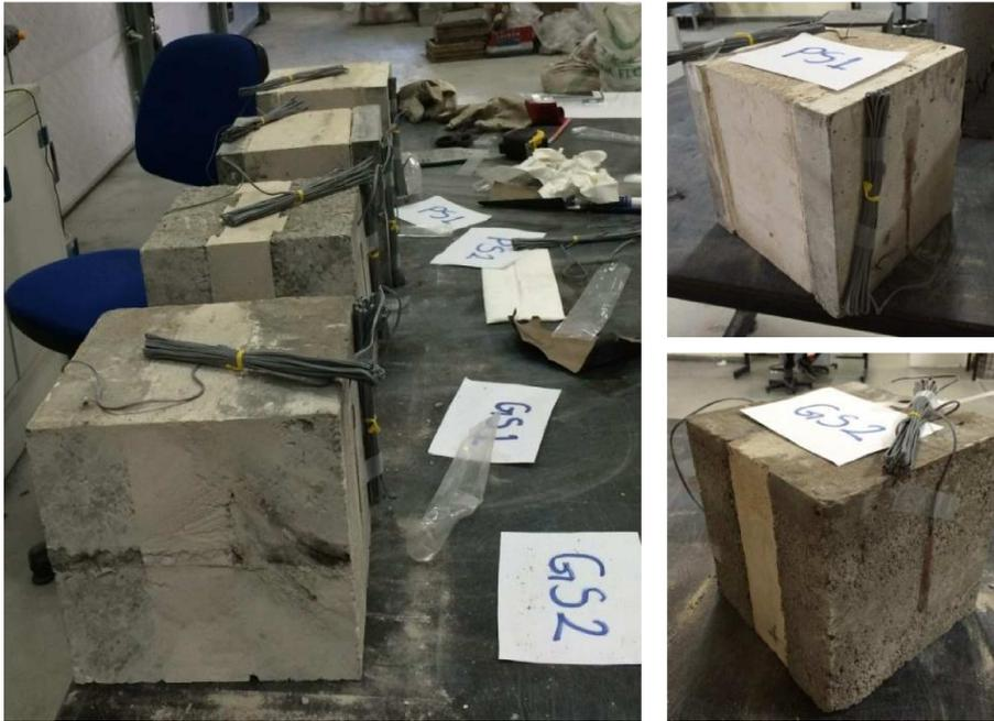
FIG. 8. Samples of grooved and plain sandwiches measured with 60 mm strain gauges.
