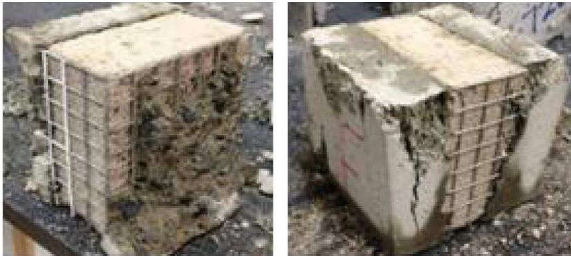
FIG. 6. Failure modes for AAC-sandwich specimens:
