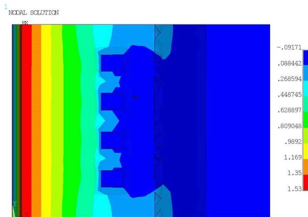
FIG. 24. The displacement image of pile cross-section of  $2.5 \times 3.5$  m.
