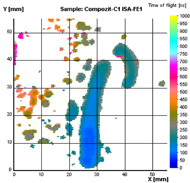
FIG. 7. Ultrasonic image in time of flight.
