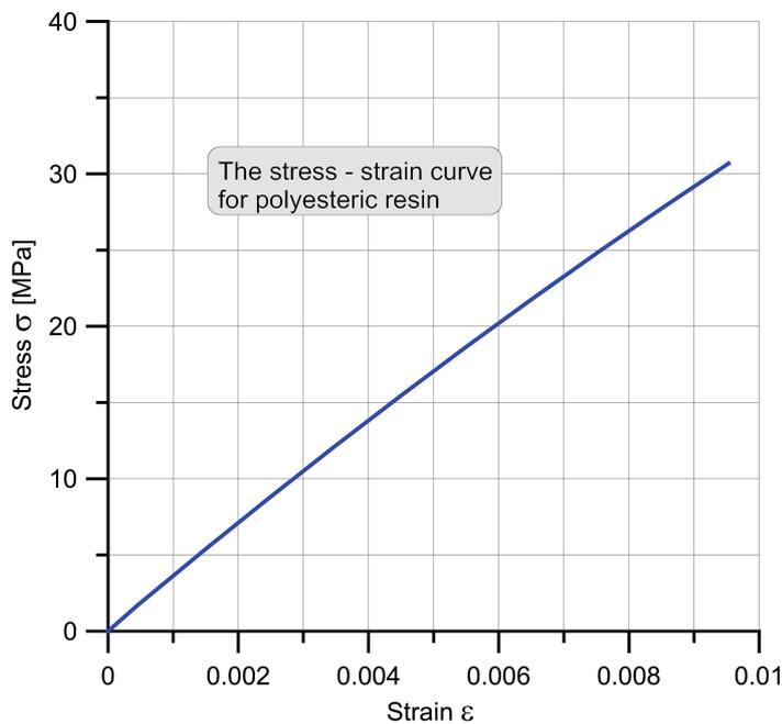
FIG. 9. The average stress-strain curve of the polyesteric resin.
