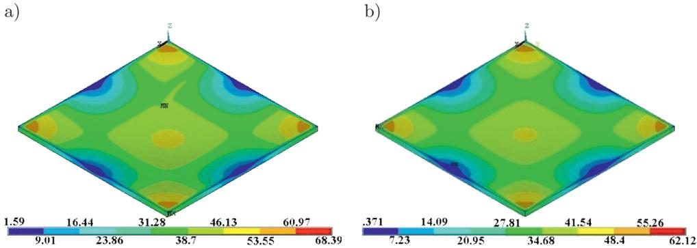
FIG. 11. Contour map of the non-dimensional von Mises equivalent stress: a) flawed plate, b) calibration plate.
