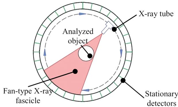
FIG. 2. Working principle of the CT scan.
