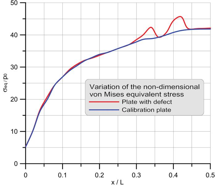
FIG. 12. Comparative variation of the von Mises equivalent stress in the middle section on line MN.
