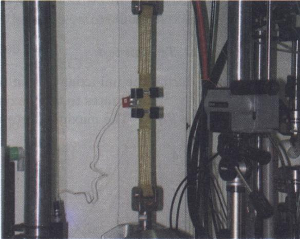
FIG. 3. Photograph of the measurement set-up designed for investigation of polyamide woven belt.
