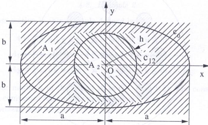
FIG. 2. Elliptic cross-section reinforced by a circular inclusion.
