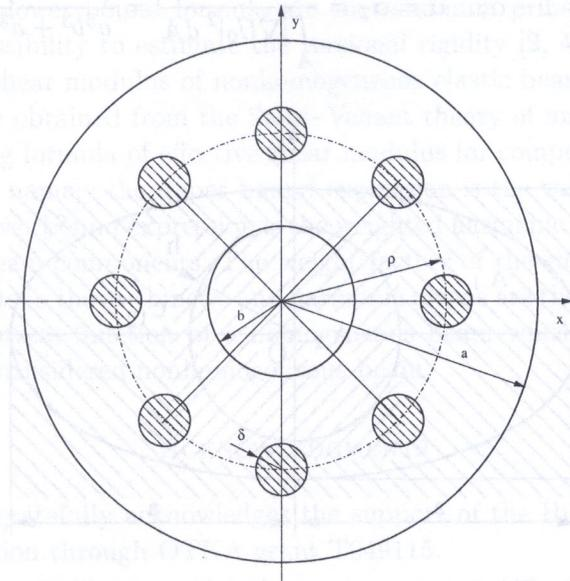
FIG. 1. Circular tube having a ring of circular inclusions.
