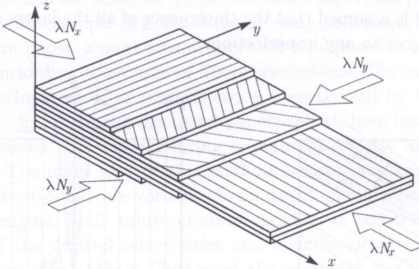
FIG. 3. Plate loading scheme.
