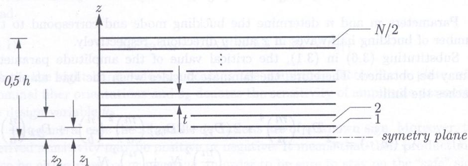
FIG. 4. Laminate cross-section.
