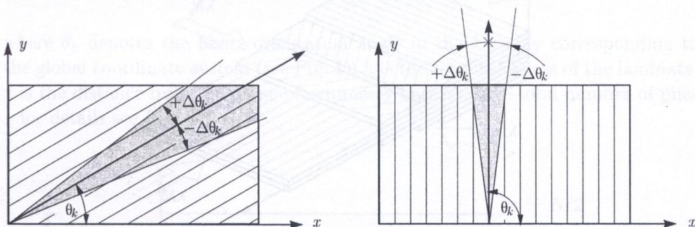
FIG. 2. Tolerances of fibers' orientations. The actual fibers' orientation stays within the allowable range  $(\theta_k - \Delta\theta_k, \theta_k + \Delta\theta_k)$ .
