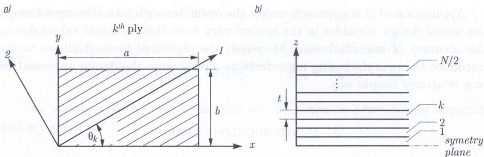
FIG. 1. Laminated sandwich plate.
