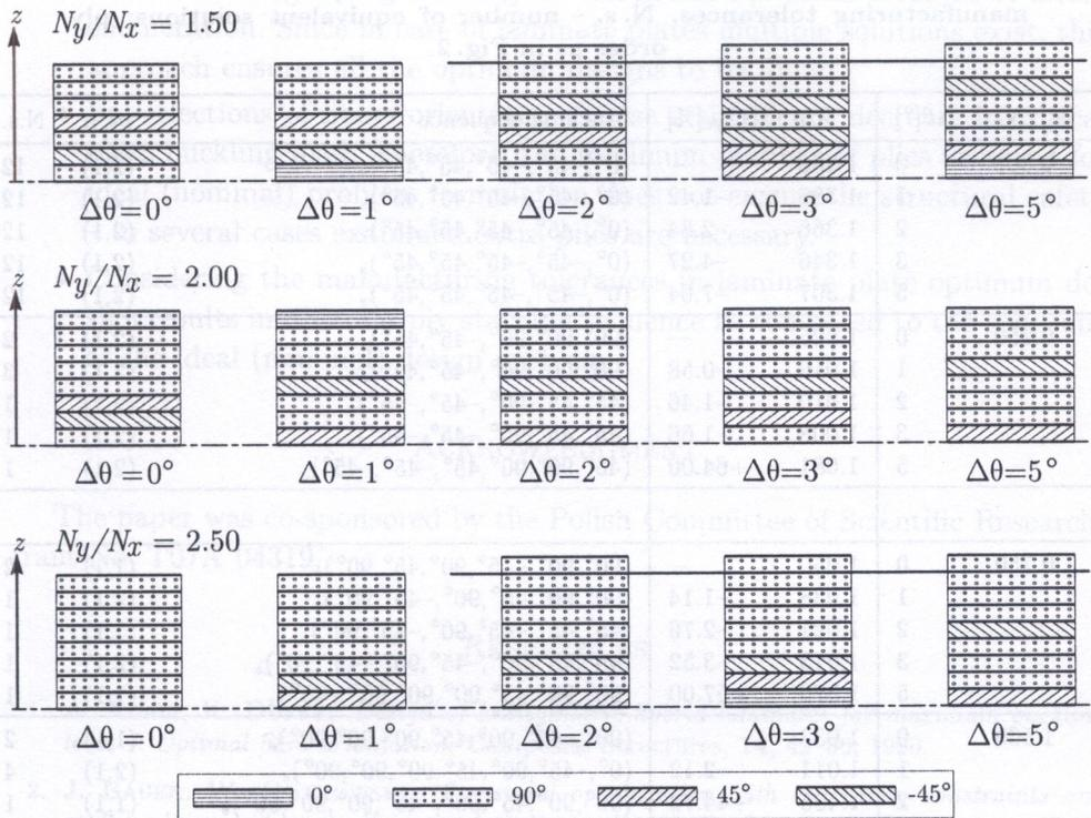
FIG. 5. Examples of ply stacking sequence in optimal laminate plates according to fiber orientation tolerances. For  $N_y/N_x = 1.5$  and  $N_y/N_x = 2.5$  extra plies are necessary if  $\Delta\theta \geq 2^\circ$ .
