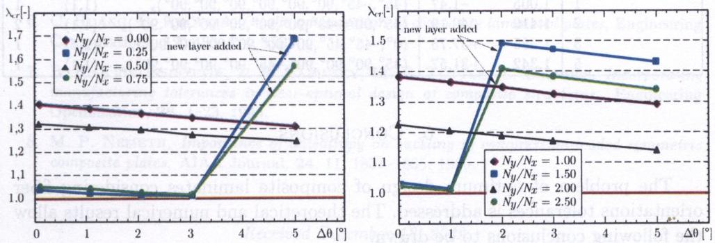
FIG. 6. Amplitude load parameter  $\lambda_{cr}$  for optimal plates considering fiber tolerances  $\Delta\theta$ .
