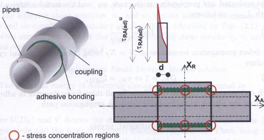
FIG. 1. Pipe-to-pipe adhesive connection: 3D and 2D views.
