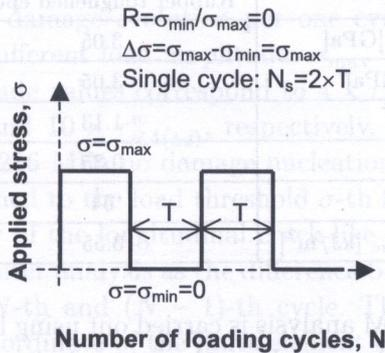
FIG. 2. Applied fatigue load.
