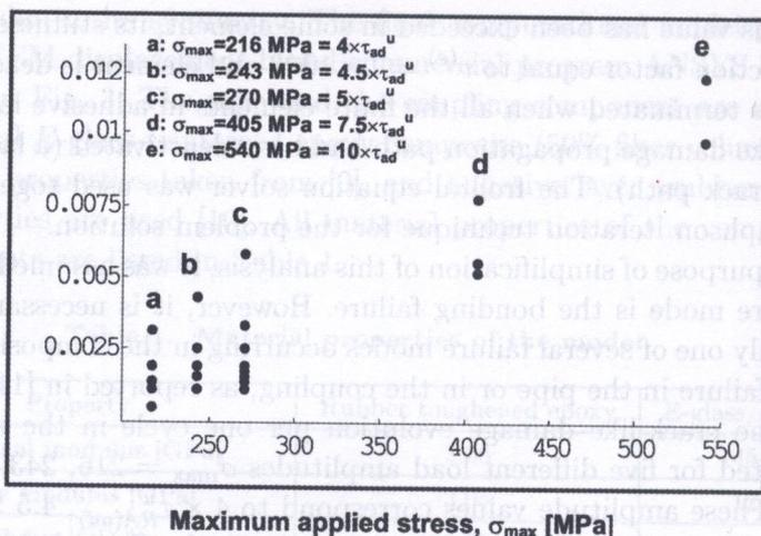
FIG. 4. Crack-like damage growth per cycle.
