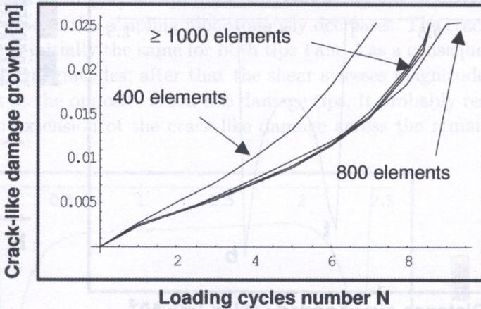
FIG. 11. Joint life sensitivity to the finite elements number in adhesive layer (vertical direction).
