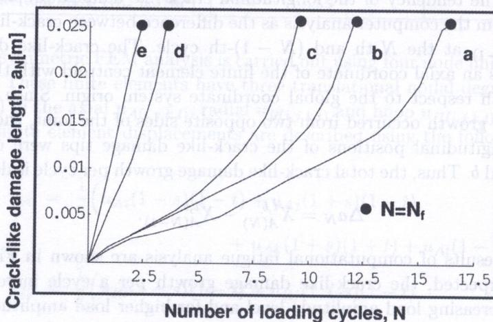
FIG. 5. Cumulative crack-like damage growth.
