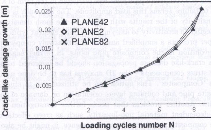
FIG. 13. Joint life sensitivity to the finite elements type in adhesive layer.
