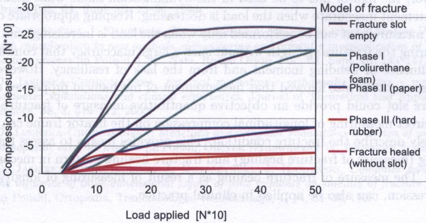
FIG. 10. Hysteresis loops of compression measured on the frame under the load applied for 5 models of fracture strength.
