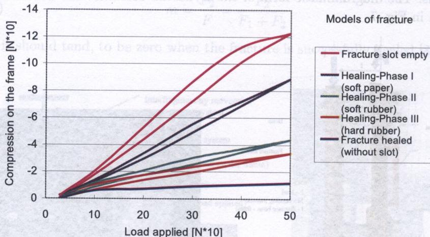
FIG. 8. Hysteresis loops of compression measured on the frame under the load applied for 5 models of fracture strength.
