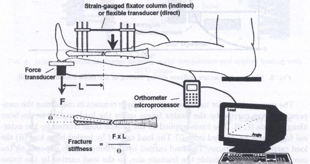
FIG. 2. Direct method of fracture stiffness measurement, after [3].
