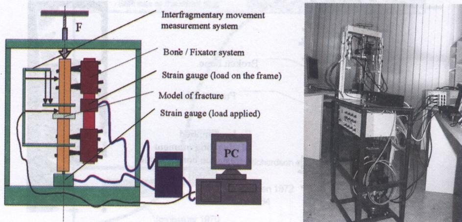
FIG. 6. Diagram of test equipment and testing machine.
