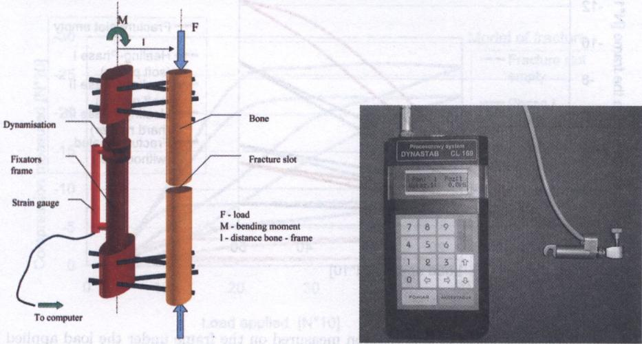
FIG. 7. Diagram of Dynastab Mechatronika 2000 external fixator showing major components and applied loading with photo of the disconnectable strain gauge.
