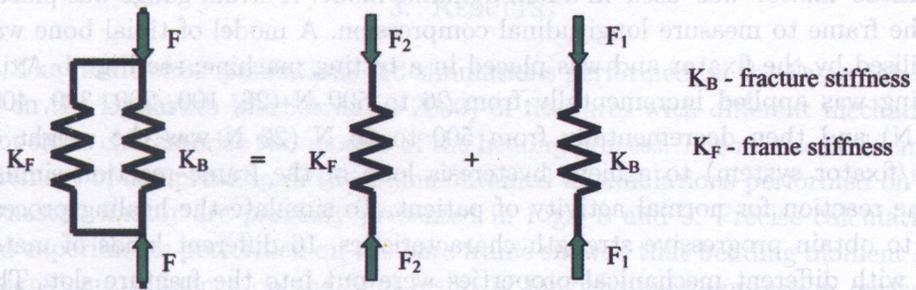
FIG. 5. Diagram of idealised fixator system as a two-spring system.
