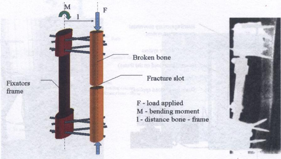
FIG. 4. Diagram of external fixator showing major components and applied loading with RTG photo.
