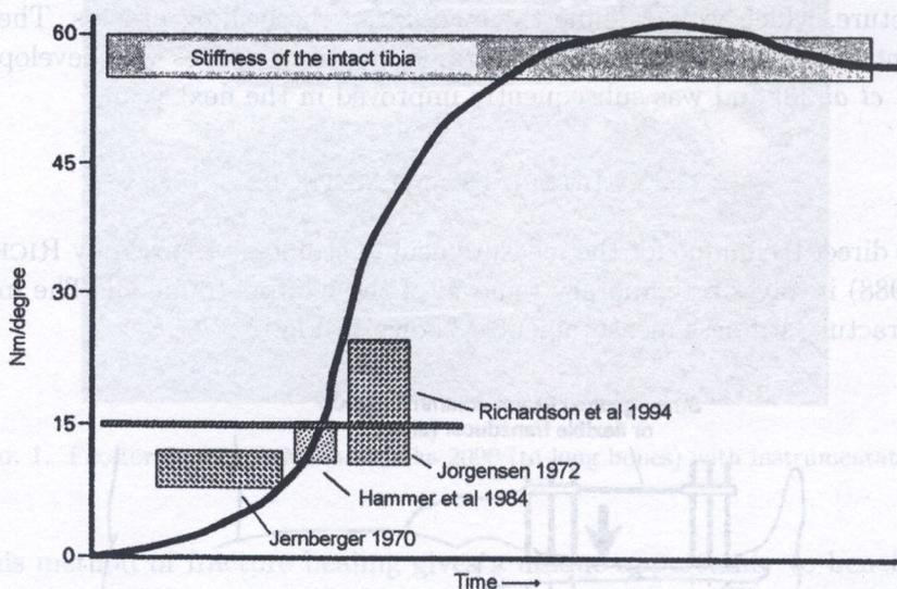
FIG. 3. Changes in fracture stiffness during healing of the tibial fractures, after [3].
