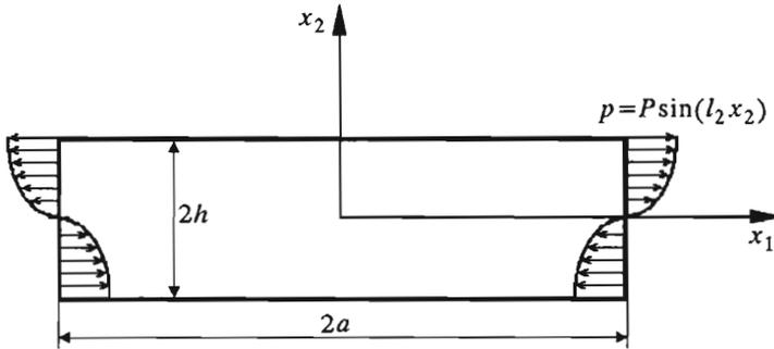
FIG. 1. Scheme of bending of a rectangular beam.
