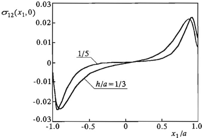
FIG. 9. Distribution of the tangential stress over the middle surface of a short beam.
