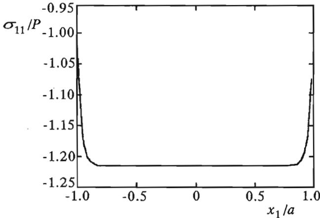
FIG. 5. Change of the normal stress  $\sigma_{11}$  on the lower surface of a beam.
