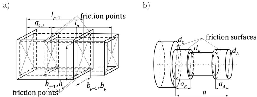
FIG. 3. Geometrical parameters of revolute (a) and prismatic (b) joint.
