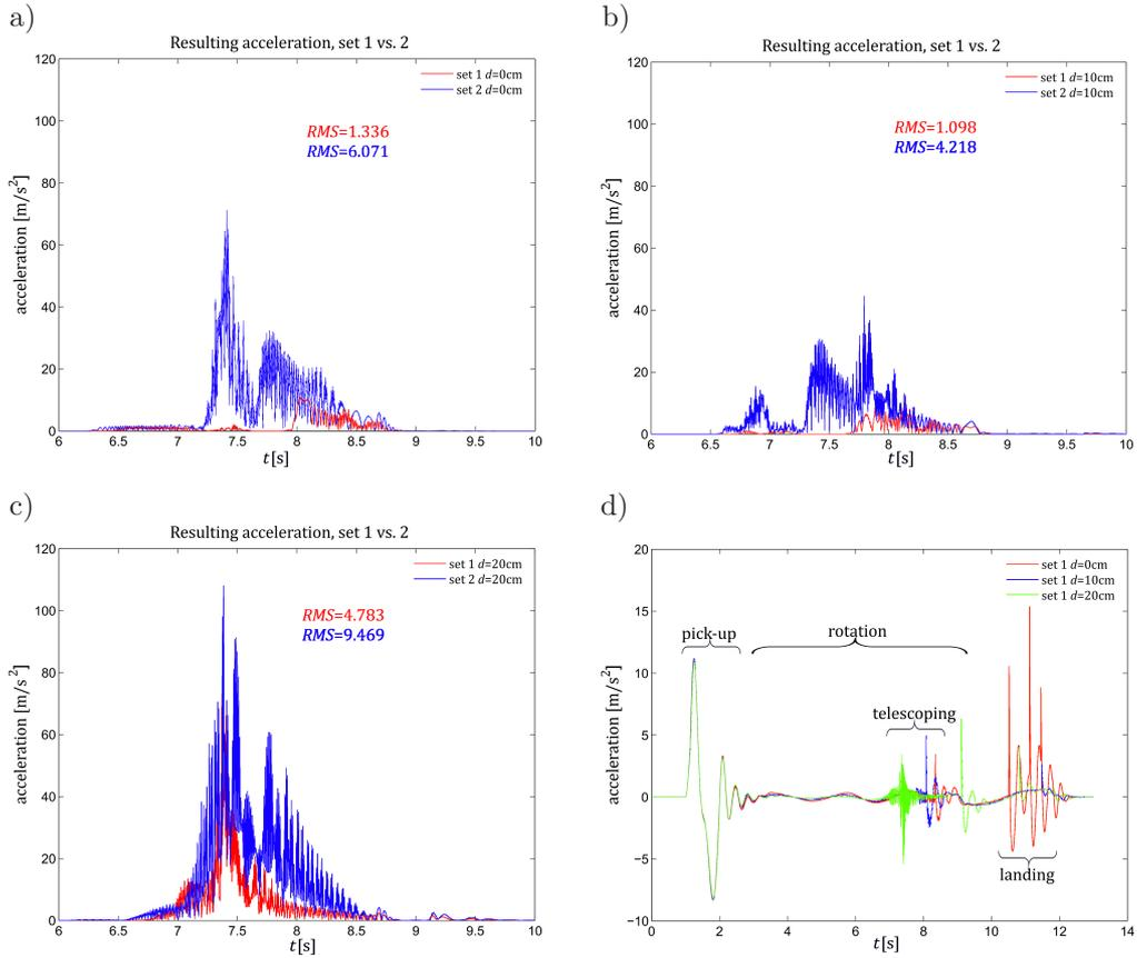
FIG. 4. Resulting acceleration on seat support for two different friction sets (a)–(c) and vertical acceleration on the body  $c_7$  CoG location (d).
