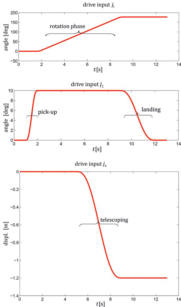
FIG. 2. Drive functions, joints  $j_1$ ,  $j_2$ ,  $j_4$ .
