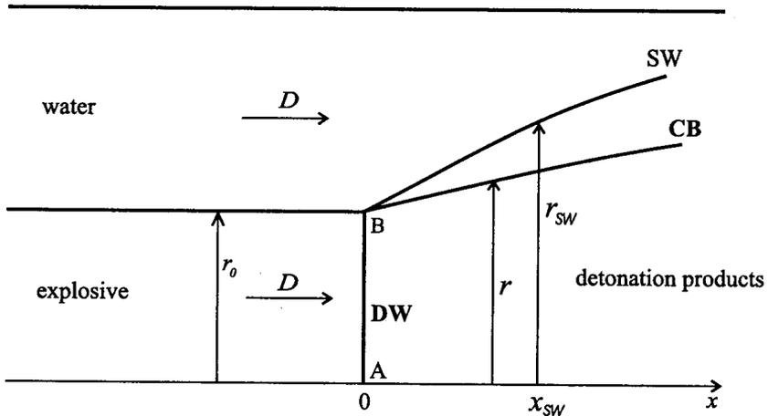
FIG. 4. Diagram of the system investigated numerically.
