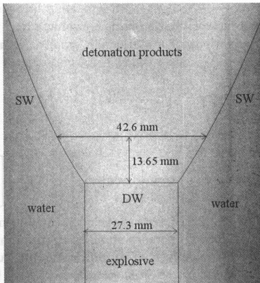
FIG. 3. An exemplary X-ray photograph of the initial stage of acceleration of a cylindrical layer of water.
