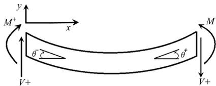
FIG. 1. Sign convention for shear forces, bending moments and slopes of the Euler-Bernoulli beam.
