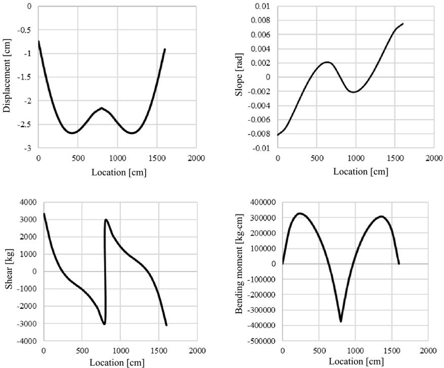
FIG. 6. Displacement, slope, bending moment, shear force of Euler-Bernoulli beam on Winkler foundation under uniformly distributed load.
