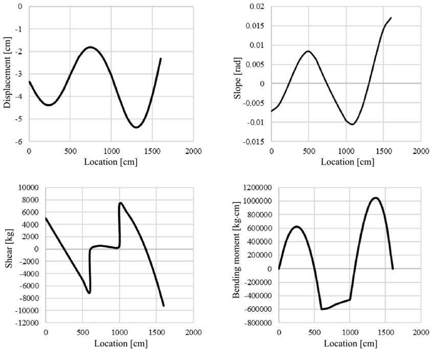
FIG. 9. Displacement, slope, bending moment, shear force of Euler-Bernoulli beam with general boundary conditions partially supported on Winkler foundation under uniformly and linearly distributed load.
