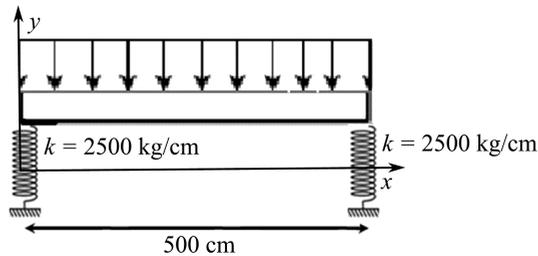
FIG. 2. Euler-Bernoulli beam under with translational restraint supported under uniformly distributed load.
