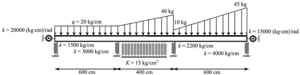
FIG. 8. Euler-Bernoulli beam with general boundary conditions partially supported on Winkler foundation under uniformly and linearly distributed load.
