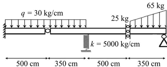
FIG. 3. Euler-Bernoulli beam with arbitrary boundary conditions under uniformly and linearly distributed load.
