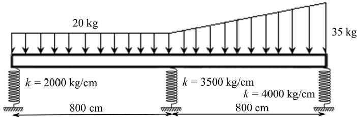
FIG. 4. Indeterminate beam under uniformly and linearly distributed load.
