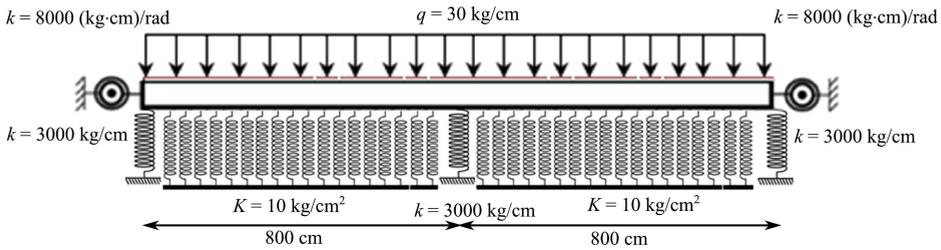
FIG. 7. Euler-Bernoulli beam with the translational and rotational support on Winkler foundation under uniformly distributed load.
