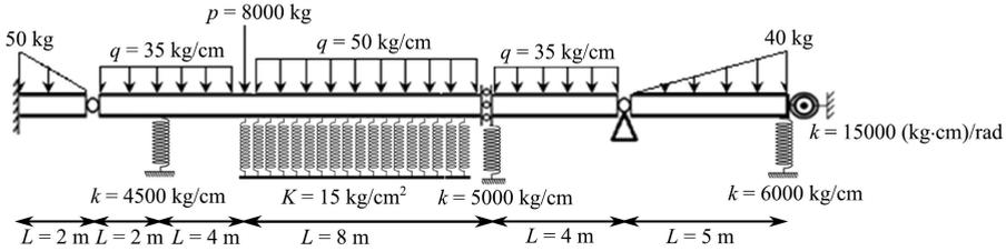
FIG. 10. Euler-Bernoulli beam with general boundary conditions partially supported on Winkler foundation under uniformly, linearly distributed and point loads.
