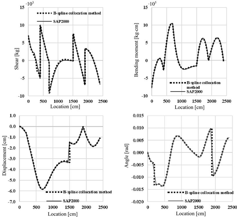
FIG. 11. Displacement, slope, bending moment, shear force of Euler-Bernoulli beam with general boundary conditions partially supported on Winkler foundation under uniformly, linearly distributed and point loads.
