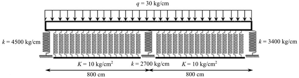
FIG. 5. Euler-Bernoulli beam on Winkler foundation under uniformly distributed load.
