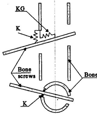
FIG. 4. Model of interaction between the bone screw and the bone.
