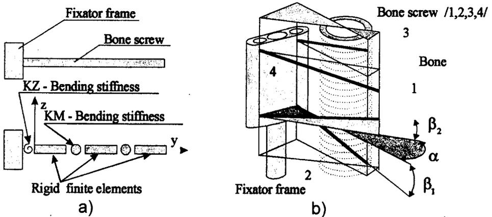
FIG. 3. a) Nominal model of the bone screws, b) Nominal model of the external fixator-bone system.
