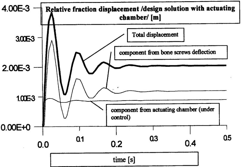
FIG. 11. Transient state (vertical load by weight of patient – 400 [N]).
