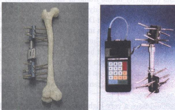
FIG. 2. Dynastab-DK fixator with the measuring circuit for healing fractures of long bones: a) version with on-board computer; b) modified version with external computer.
