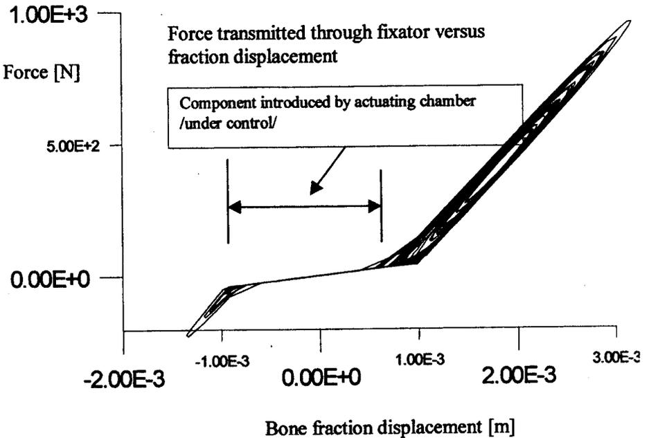
FIG. 12. Hysteresis caused by vertical load from – 50 to 1000 [N].
