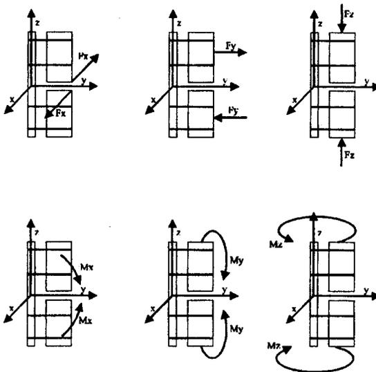
FIG. 5. Analysed types of loads in the external fixator-bone system.
