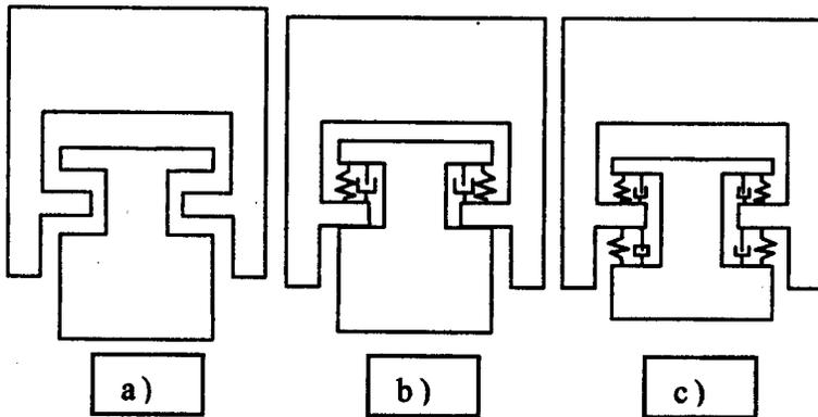
FIG. 10. Designs of dynamising chambers: a) two-directional with clearance, b) one-directional with flexible element, c) two-directional with flexible element (applied in Dynastab-DK fixators).
