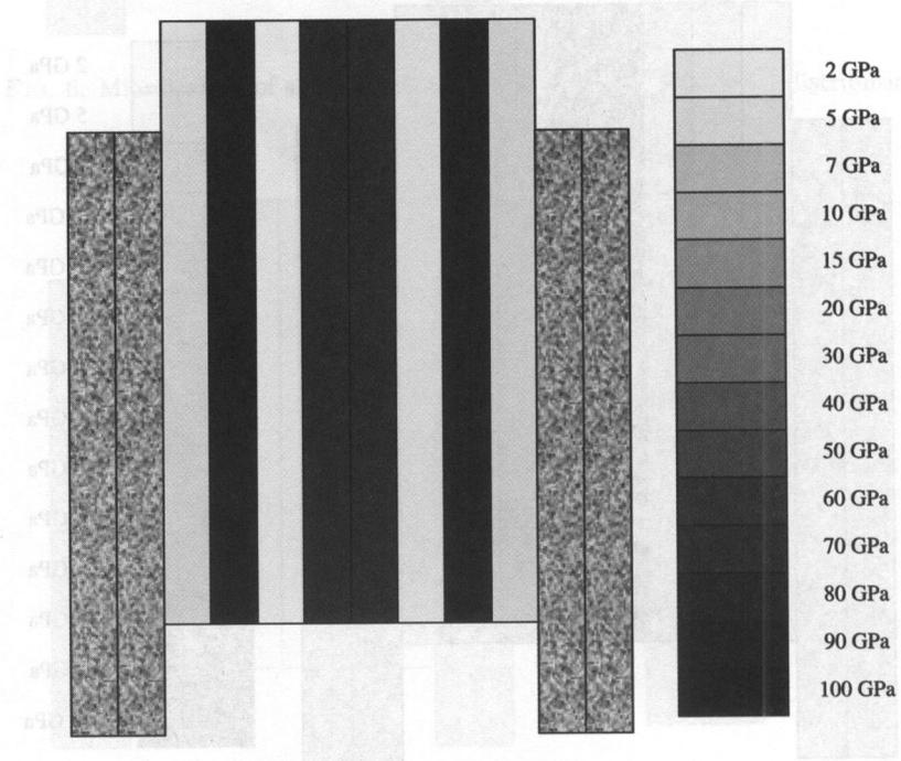
FIG. 11. Minimization of shear stress  $\sigma_{xy} \rightarrow \min$  subject to the constraint  $m_r < m_0$ . Optimal material distribution.
