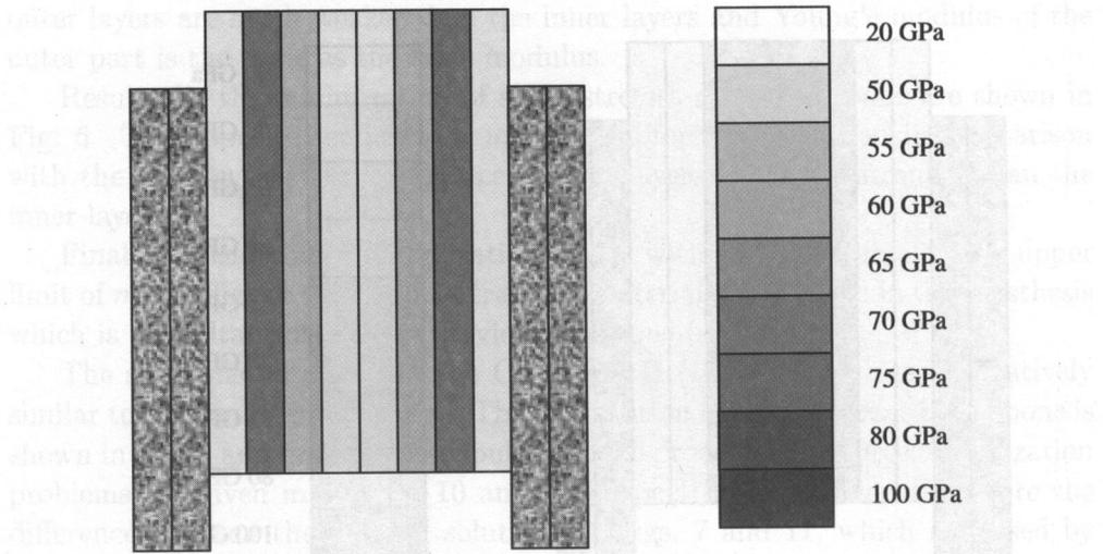
FIG. 7. Minimization of shear stress  $\sigma_{xy} \rightarrow \min$  subject the constraint  $m_r < m_0$ . Optimal material distribution.
