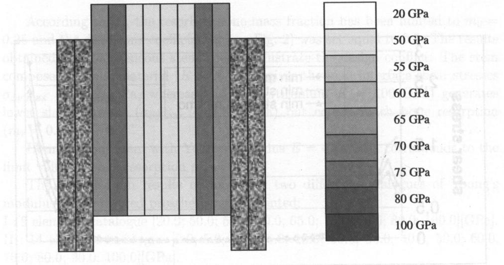
FIG. 6. Minimization of shear stress  $\sigma_{xy} \rightarrow \min$ . Optimal material distribution.
