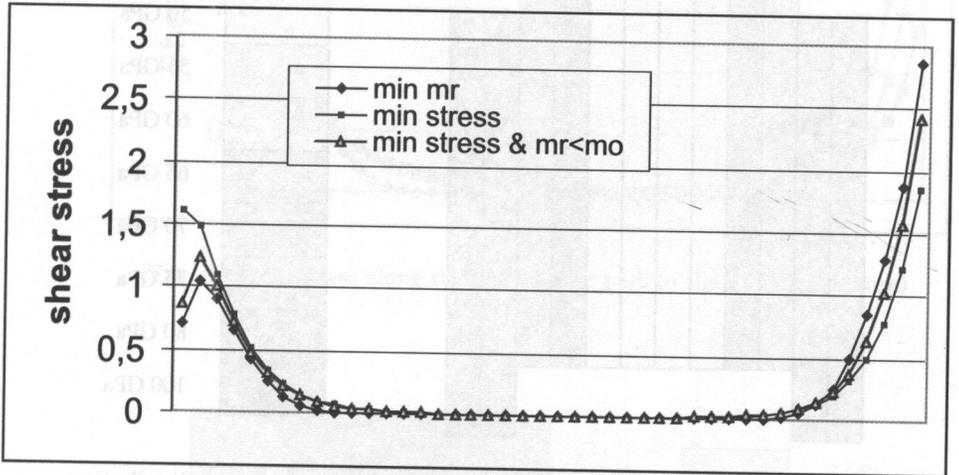
FIG. 4. Shear stress along the bone (lower part to the left of the figure).
