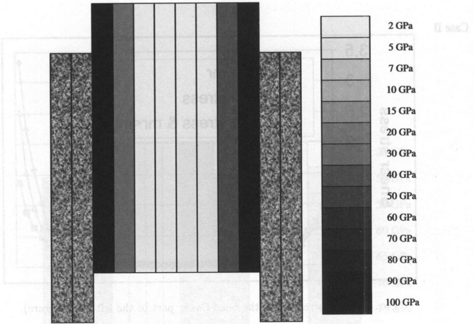
FIG. 10. Minimization of shear stress  $\sigma_{xy} \rightarrow \min$ . Optimal material distribution.
