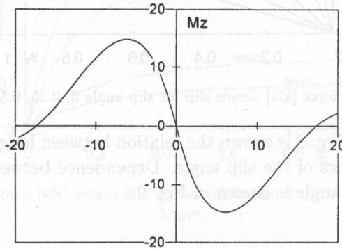
FIG. 9. Self-aligning moment [Nm] versus slip angle [deg] for pure cornering ( $s_x = 0$ ).
