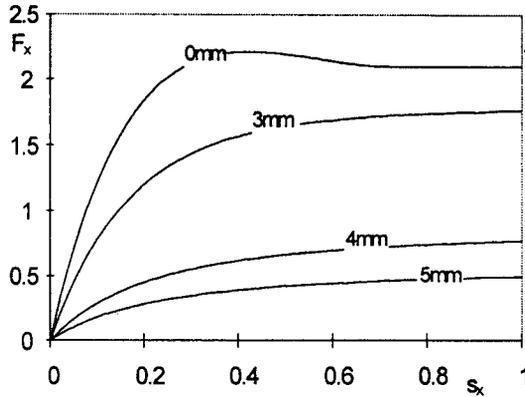
FIG. 4. Longitudinal force [kN] versus slip  $s_x$  for thickness of the water film  $h_0 = 0, 3, 4$  and 5 mm.
