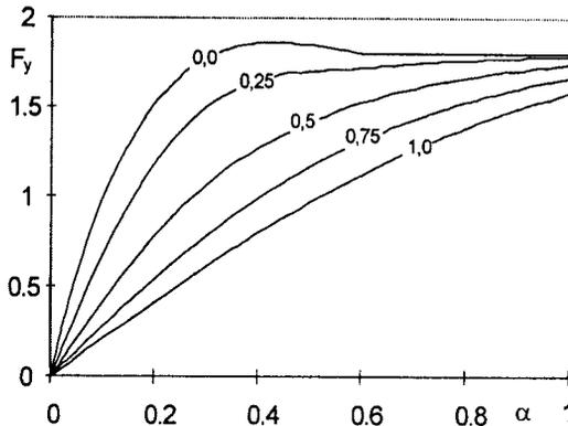
FIG. 7. Lateral force [kN] versus slip angle [rad] for slip  $s_x = 0, 0.25, 0.5, 0.75$  and 1.0.
