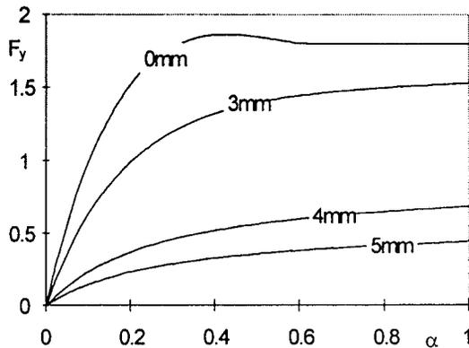
FIG. 5. Lateral force [kN] versus slip angle  $\alpha$  for thickness of the water film  $h_0 = 0, 3, 4$  and 5 mm.
