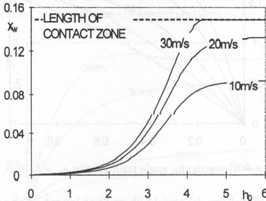
FIG. 10. Length of the water zone [m] versus thickness of the water film [mm] for velocity  $v_x = 10, 20$  and  $30$  m/s.
