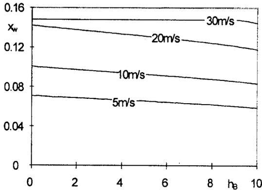
FIG. 11. Length of the water zone [m] versus height of the tread elements [mm] for velocity  $v_x = 5, 10, 20$  and  $30$  m/s.
