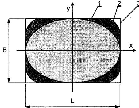
FIG. 2. Shape of the contact zone; 1 – elliptic; 2 – real; 3 – rectangular.
