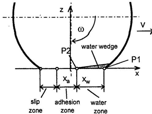
FIG. 1. Contact zones of the tire model.
