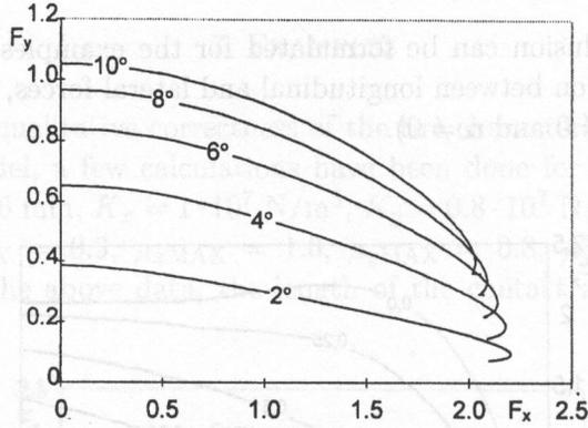
FIG. 8. Lateral force [kN] versus longitudinal force [kN] for slip angle  $\alpha = 2^\circ, 4^\circ, 6^\circ, 8^\circ$  and  $10^\circ$ .
