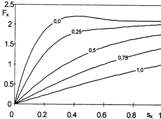
FIG. 6. Longitudinal force [kN] versus slip for slip angle 0, 0.25, 0.5, 0.75 and 1.0 rad.
