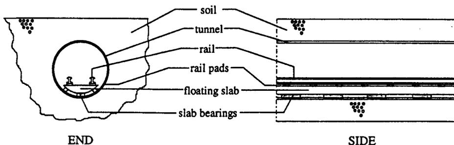
FIG. 1. The layout of floating-slab track for underground railway lines.
