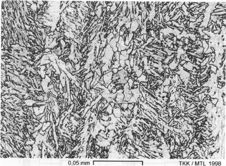
FIG. 2. Microstructure of fusion zone for grade A steel.
