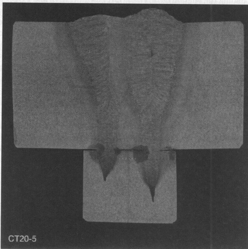
FIG. 1. Etched macrosection of  $20 \times 15$  stake weld.
