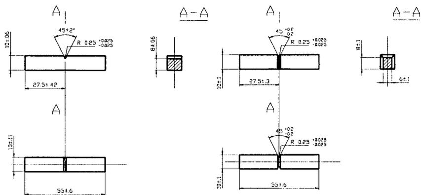
FIG. 3. Standard and modified (3-notch) Charpy specimen.
