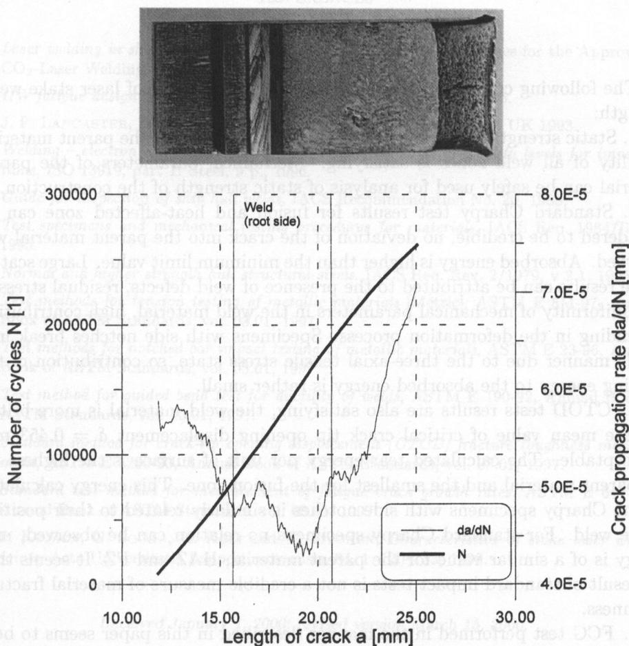
FIG. 8. Example of FCG test result and fracture appearance.
