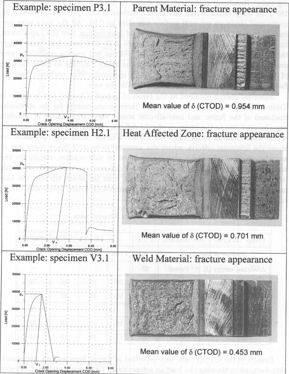
FIG. 7. Examples of load-COD plots and fracture appearance for PM, HAZ and FZ.
