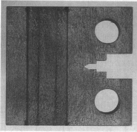
FIG. 5. Compact specimen with transversal weld (root side of the weld).
