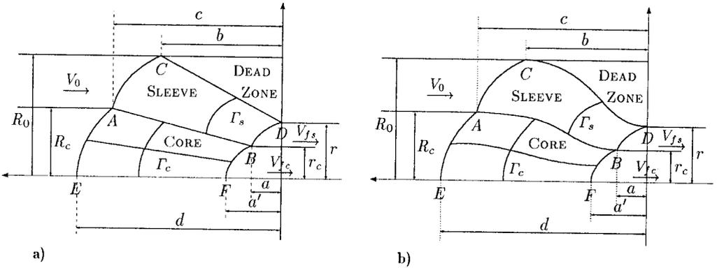
FIG. 1. General concept of the flow field construction in extrusion of bimaterial system: flow lines are straight a) or smooth b).
