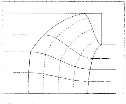
FIG. 3. Plastic zone and flow lines for both different models for Pb/OT3 composite (the hard core)  $\lambda = 3$  and  $R_0/R_c = 2$ .
