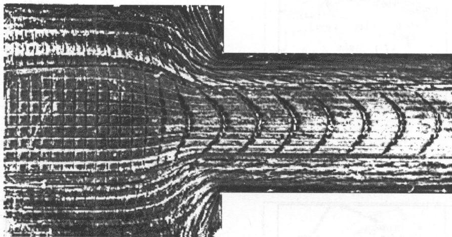
FIG. 5. Experimental grid distortion for Pb/OT3 composite (the hard core).
