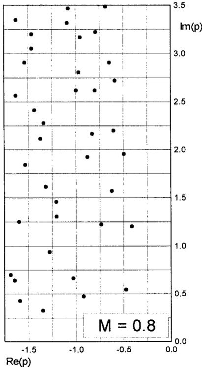
FIG. 4. Latent roots for an aspect-ratio-three rectangular wing.
