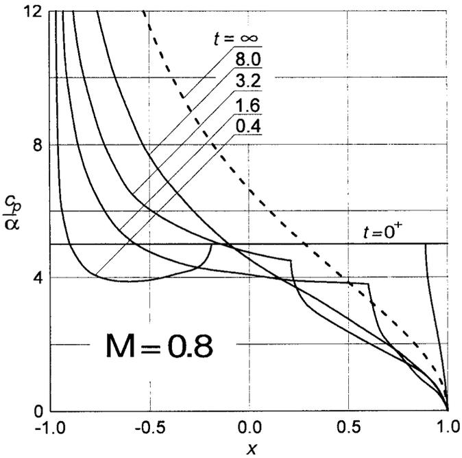
FIG. 7. Chordwise lifting pressure distributions on an airfoil. After LOMAX [23].
