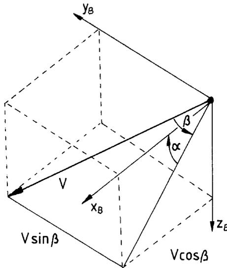
FIG. 2. Coordinates used in Flight Dynamics.
