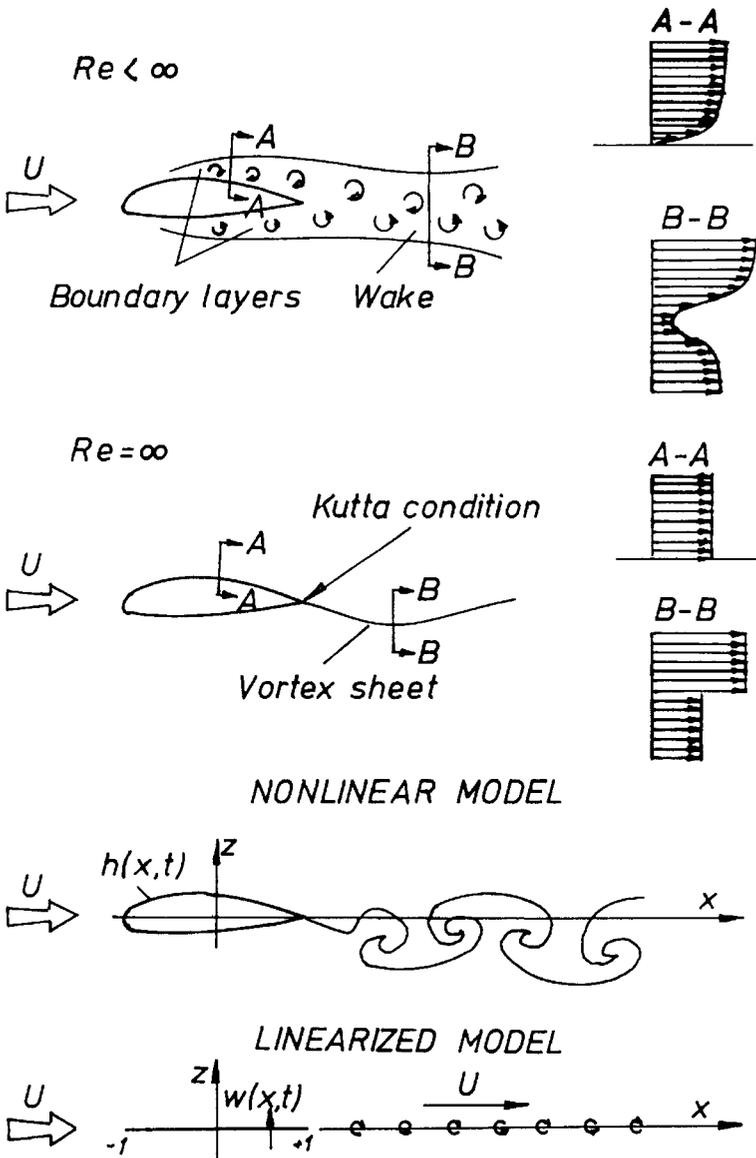
FIG. 3. The linearized unsteady aerodynamic model.
