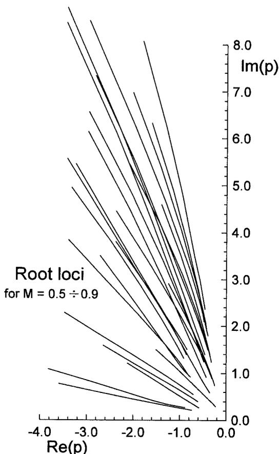
FIG. 6. Latent root loci for an aspect-ratio-three rectangular wing.
