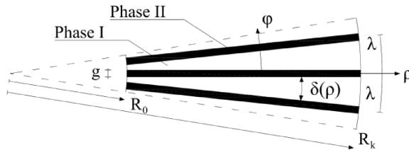
FIG. 2. Deterministic microstructure of composite.
