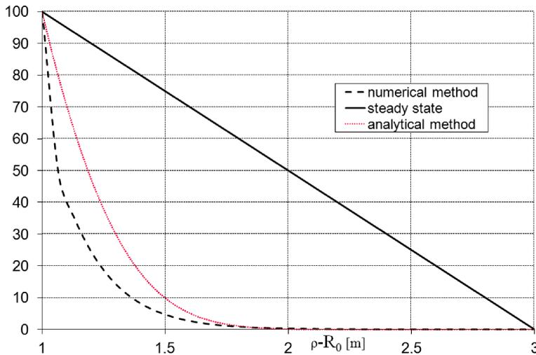
FIG. 4. The results of analytical and numerical method – Case No. I after  $t = 1$  [h]. A diagram of averaged temperature.
