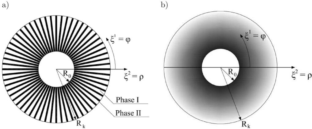
FIG. 1. Structure of two-phase functionally graded composites on a) micro- and b) macro-scale.
