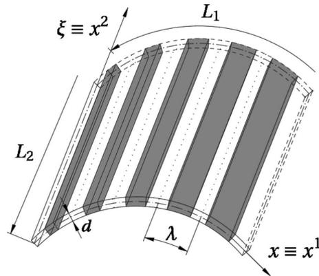
FIG. 1. An example of a shell with a tolerance-periodic microstructure.
