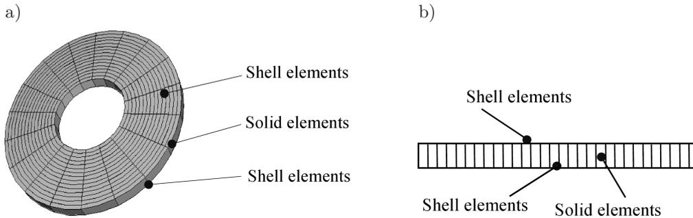
FIG. 2. FEM plate models: a) basic, b) simplistic.
