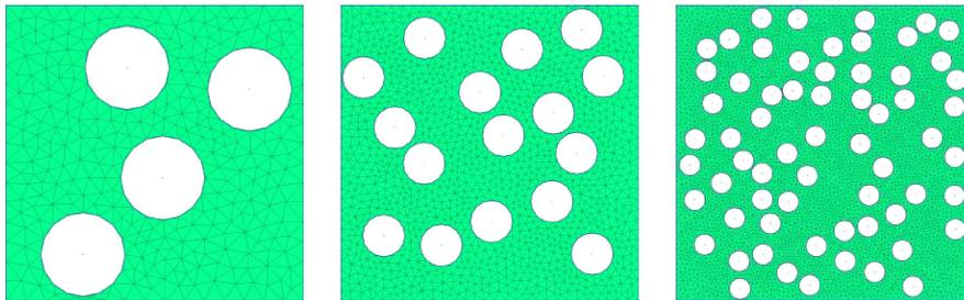
FIG. 1. Examples of the representative volume elements of the size 2, 4, 6, i.e. with 4, 16 and 64 holes, respectively. All RVEs have void ratio equal to 0.25.
