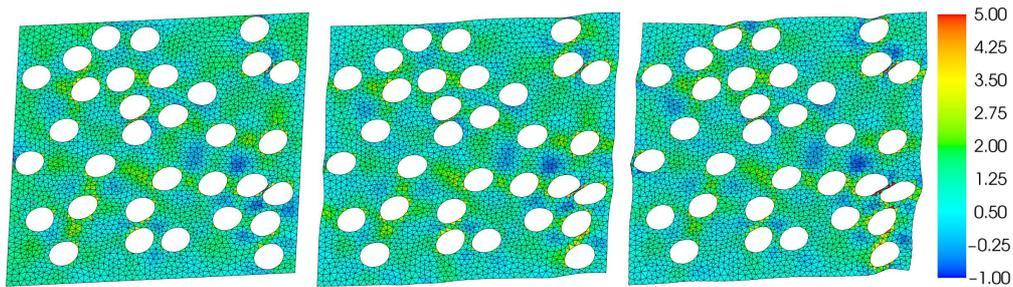
FIG. 2. Deformations (zoom 500×) and shear stresses (in kPa) for the exemplary RVE of the size 5 under different boundary conditions. From left to right: linear displacement BCs, periodic displacement BCs, minimal kinematic BCs.
