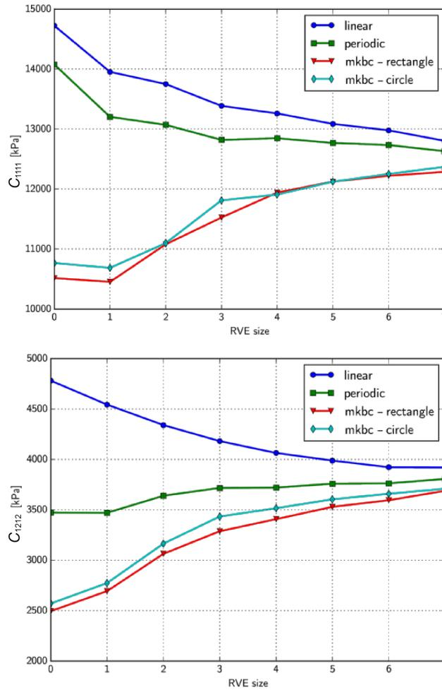
FIG. 3. Convergence of the computed elastic moduli to their effective values with increasing RVE size for different boundary conditions ( $C_{1111}$  on the top,  $C_{1212}$  on the bottom).
