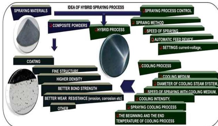
FIG. 3. Idea of hybrid spraying process.
