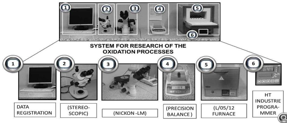
FIG. 4. Research corrosion stand.
