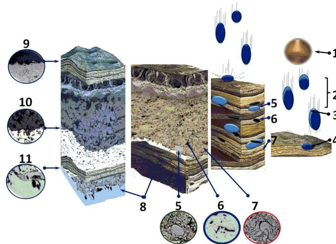
FIG. 1. Building a full coating of a desired thickness: 1 – heat source (arc, flame), 2 – speeding up particles, 3 – oxide coating, 4 – blowing particles into the ground, 5 – non-molten particles, 6 – pores, 7 – oxide layers, 8 – base material, 9 – surface roughness, 10 – transition zone in the coating layered, 11 – transition zone between the coating.
