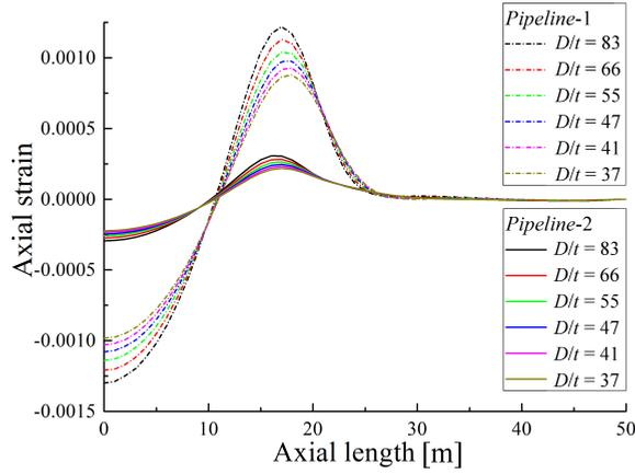
FIG. 7. Axial strain curves of the upper surface under different radius-thickness ratios.
