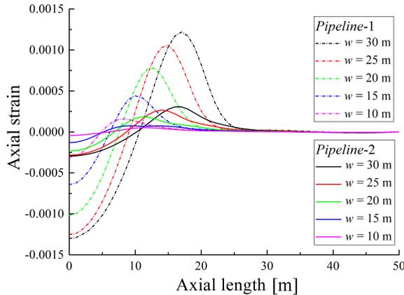
FIG. 13. Axial strain curves of the upper surface under different widths.
