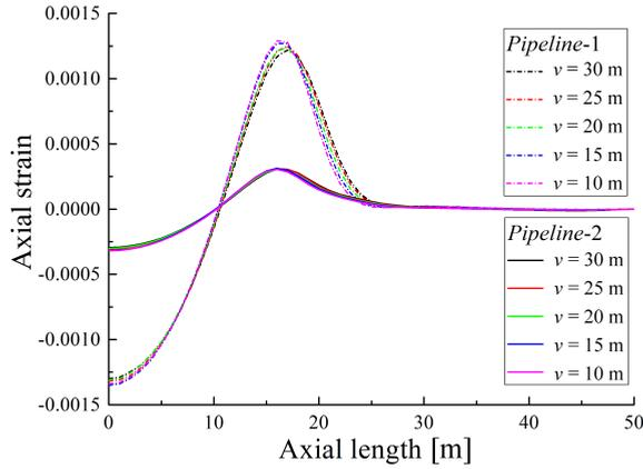
FIG. 15. Axial strain curves of the upper surface under different lengths.
