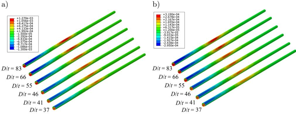
FIG. 6. Axial strain of the pipeline under different radius-thickness ratios: a) pipeline-1, b) pipeline-2.
