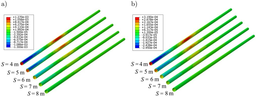
FIG. 9. Axial strain of the pipeline under different distances: a) pipeline-1, b) pipeline-2.
