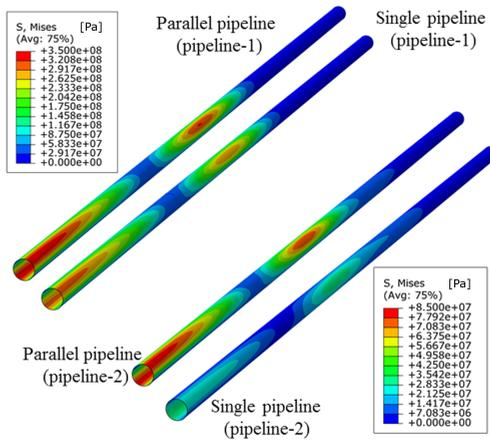
FIG. 3. Difference between parallel pipeline and single pipeline.
