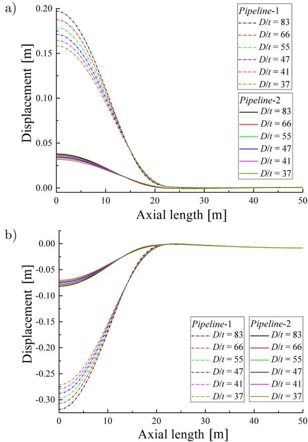
FIG. 8. Displacement of the pipeline under different radius-thickness ratios: a) horizontal displacement ( $x$ -direction), b) vertical displacement ( $z$ -direction).
