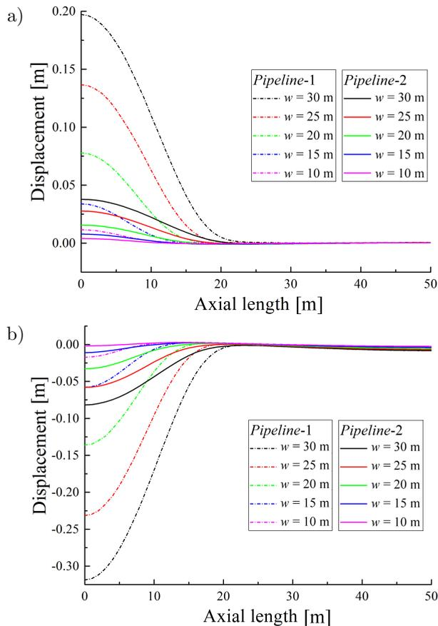
FIG. 14. Displacement of the pipeline under different widths: a) horizontal displacement ( $x$ -direction), b) vertical displacement ( $z$ -direction).
