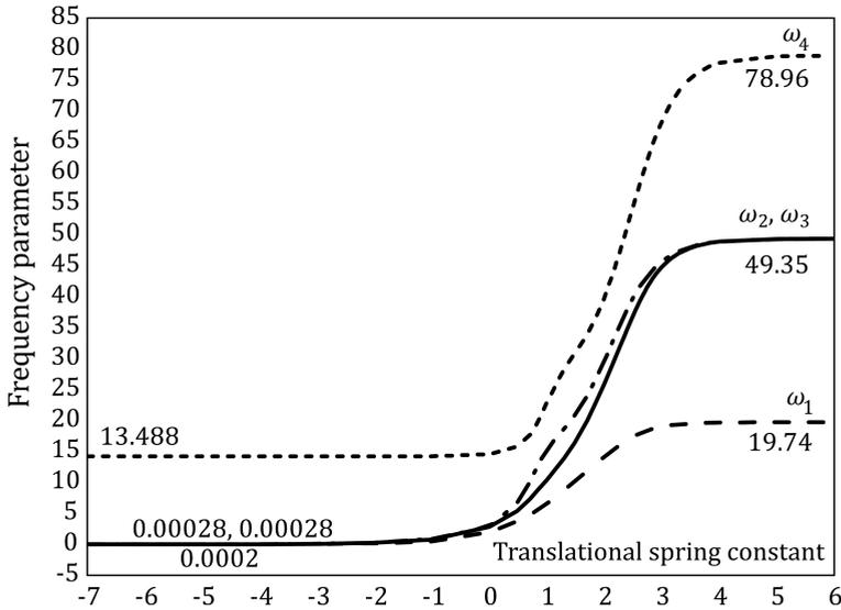
FIG. 8. Square TTTT Plate: frequency parameter as a function of translational end spring constants.
