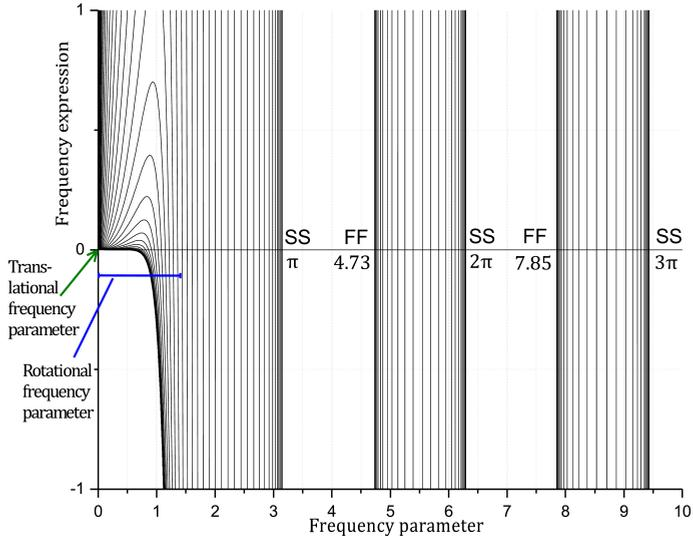
FIG. 2. Frequency expression of a beam with translational edge support at both ends (TT beam) vs. frequency parameter.
