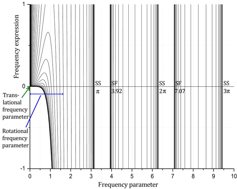
FIG. 5. Frequency expression of a beam with translational edge support at one end (ST beam) vs. frequency parameter.
