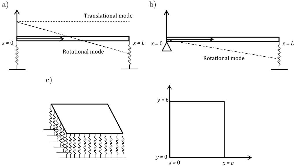
FIG. 1. a) TT beam, b) ST beam, c) elastically edge supported Kirchhoff's plate.
