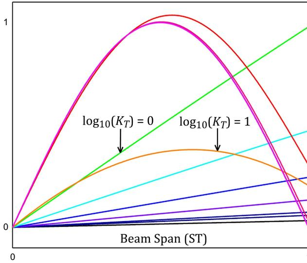
FIG. 7. Modeshape associated with the 1st frequency parameter of ST beam.
