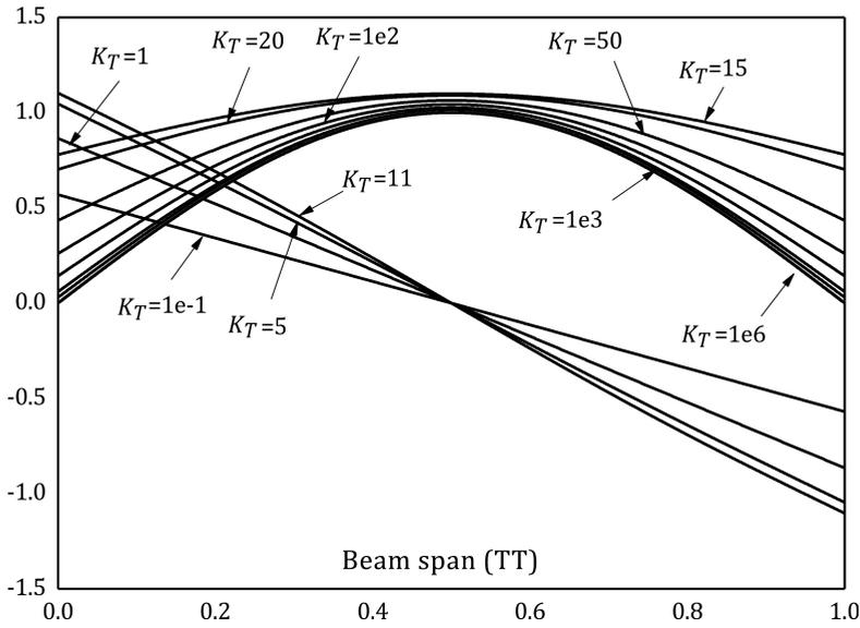
FIG. 4. Modeshape associated with the 2nd frequency parameter of TT beam: transition from rotational rigid-body modeshape of FF beam to first flexural modeshape SS beam.
