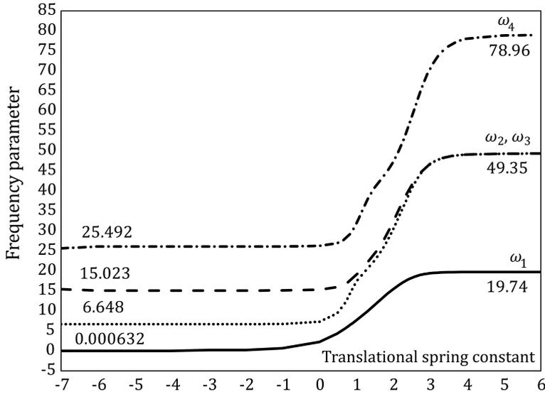
FIG. 9. Square STTT Plate: frequency parameter as a function of translational end spring constants.
