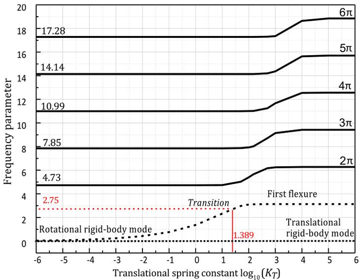
FIG. 3. TT Beam frequency parameter as a function of translational end spring constants.
