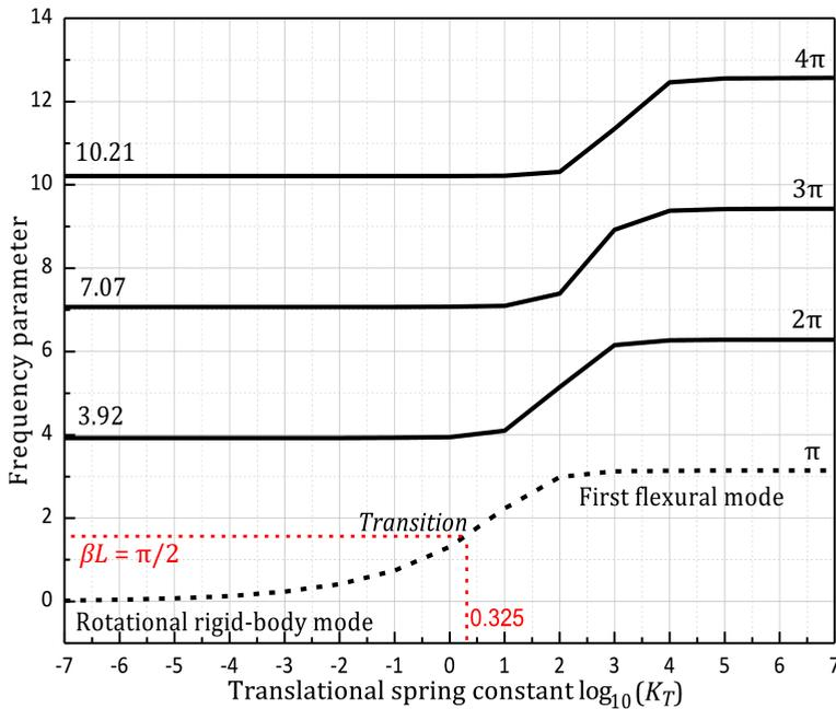
FIG. 6. ST Beam frequency parameter as a function of translational end spring constants.
