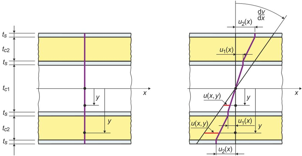
FIG. 2. The scheme of the deformation of straight line – the Zig-Zag hypothesis.
