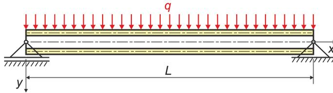
FIG. 1. Scheme of the symmetrical seven layer beam under transverse load.
