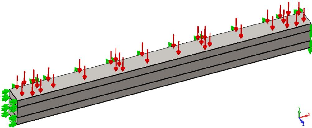
FIG. 3. The scheme of the beam with boundary conditions and load.
