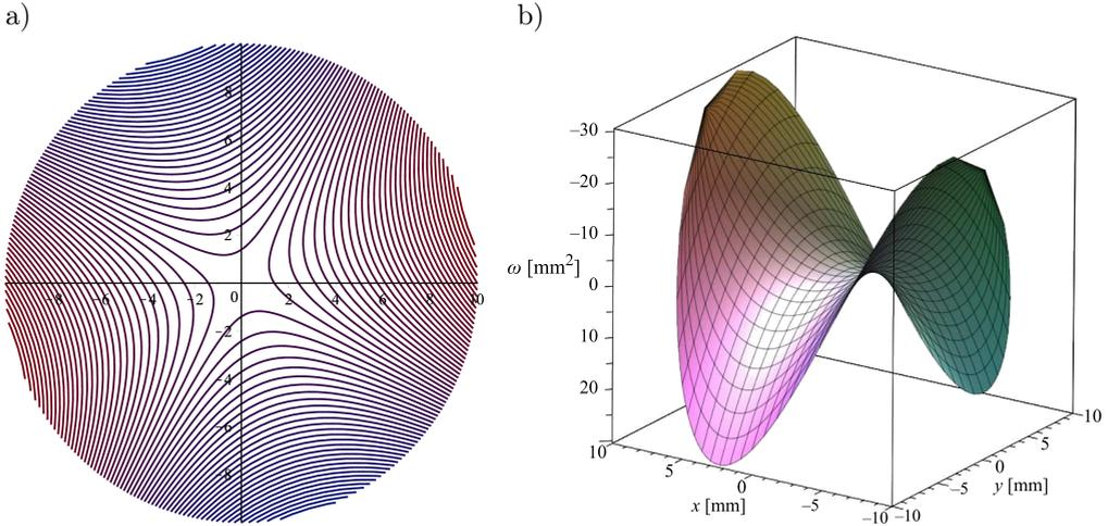
FIG. 2. Illustrations of the torsion function: a) contour lines, b) graph of the torsion function.
