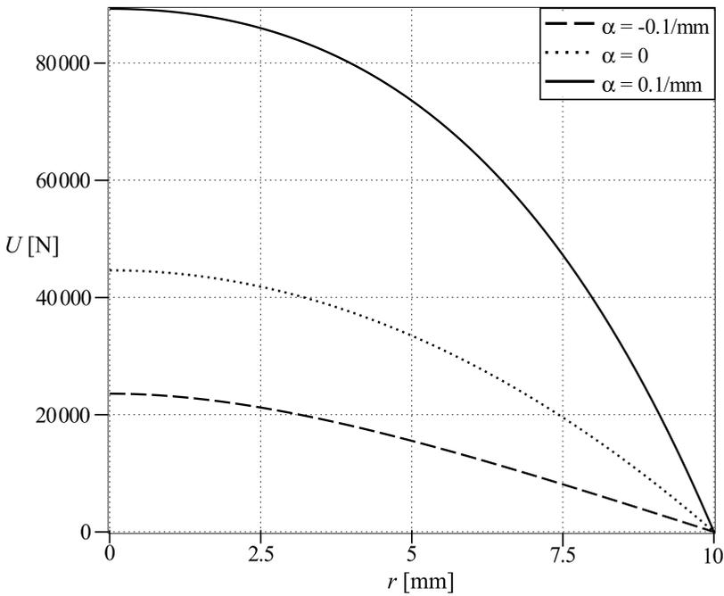
FIG. 3. The graphs of the Prandtl’s stress functions.
