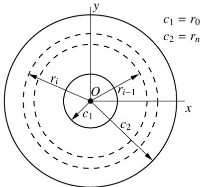
FIG. 5. Layered hollow circular cross-section.
