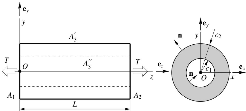
FIG. 1. Hollow circular cylinder.
