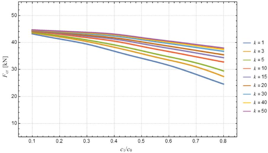
FIG. 3. The influence of  $k$  parameter and the  $c_1/c_0$  ratio on critical loads values.
