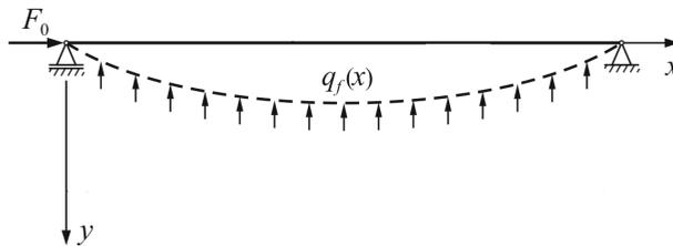
FIG. 1. The scheme of homogeneous beam.
