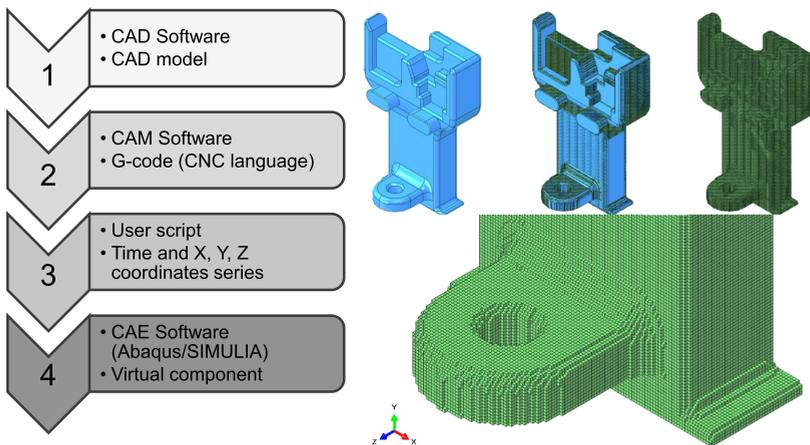
FIG. 3. Schema of the approach based on finite element analysis.
