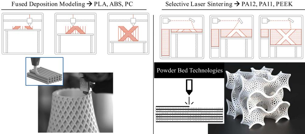
FIG. 1. Schemas of the FDM and SLS processes.
