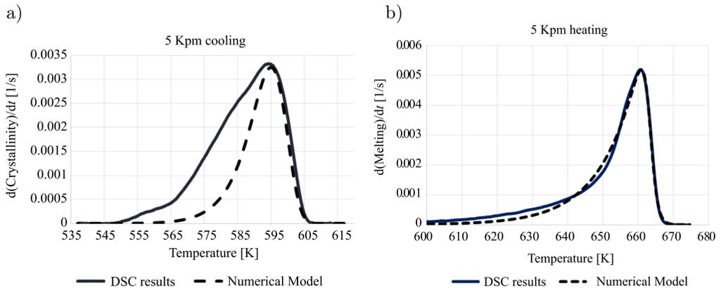
FIG. 2. a) Comparison of the model prediction with the DSC results, b) parameter adjustment of the melting model with use of the DSC results.
