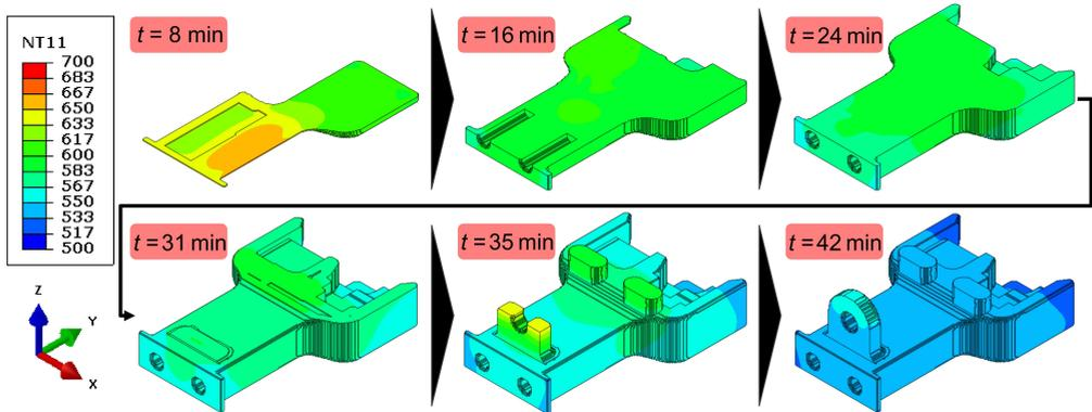
FIG. 4. Temperature [K] distribution during AM process.
