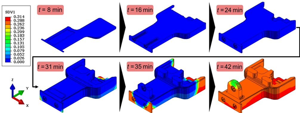
FIG. 5. Degree [-] of crystallinity during AM process.
